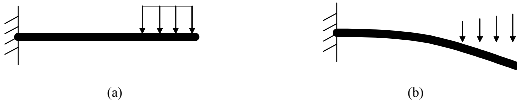
Figure 3. 25: (a) Loading state of the cantilever (b) Bending curve of the cantilever
