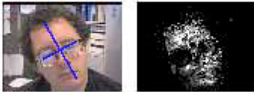
Figure 5.4: Orientation of the flesh probability distribution marked on the source video image. (Bradski, 1998)
