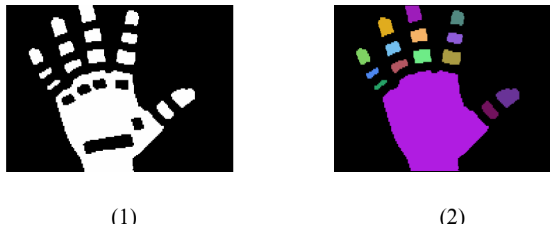
Figure 7.20: At the end of the filtering Figure 7.19-(1), the gray result image is found (1). By accepting (1) as input, the connected components are found in (2).
