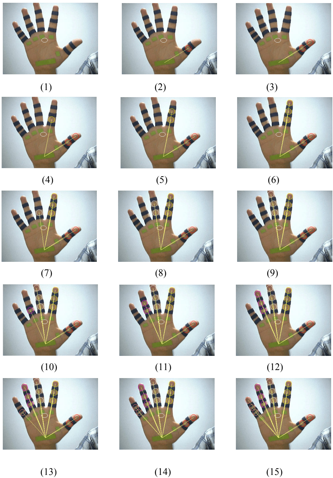
Figure 7.22: Hand regions are found and labeled in order (according to the reference green point )
