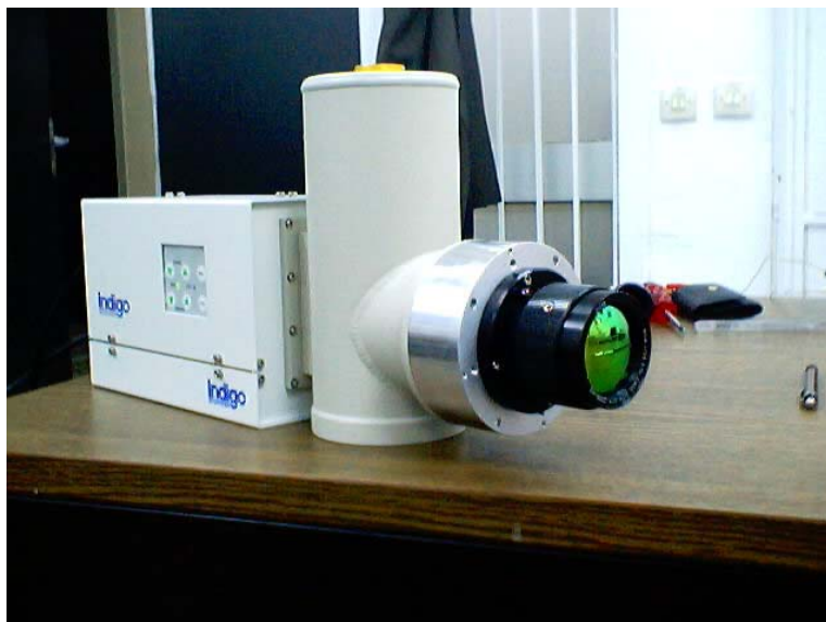
Figure 5.11: Indigo Systems' ISC9801 Standard 128 evaluation camera [49].
