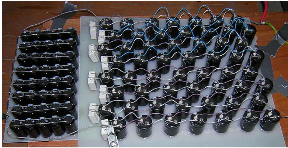
Figure 4.4: Capacitor bank of the DC power supply has a capacitance of 150 \mu F, maximum voltage of around 3000VDC.
