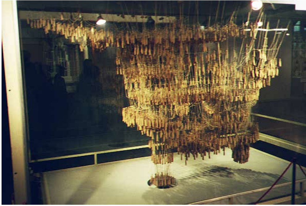
Figure 3.17. Rope & Case Model of Sagra da Familia
