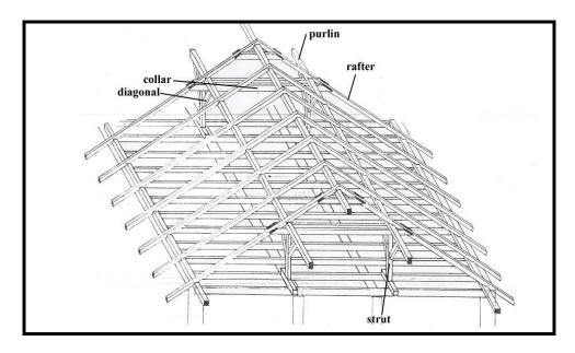
Figure II. 12 Two purlin hip roof is composed of rafters, purlins, diagonals, collars and struts. The ridge purlin is placed for easy installation (Binan, 1990:78).
