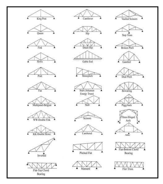
Figure II. 26 Typical truss types have various names in different cultures (Faherty, 1989: 6.7-6.8).
