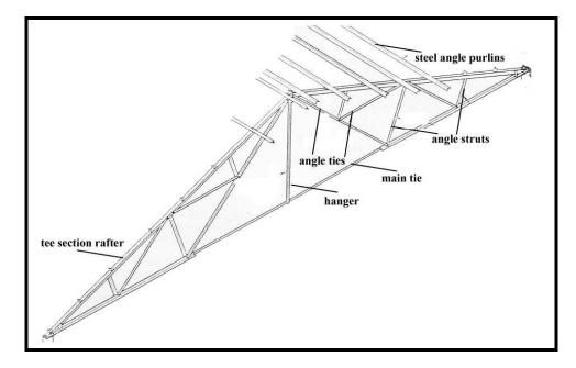
Figure II. 30 Steel trusses are composed of rafters, purlins, hangers, struts and ties (Foster, 1983:346).
