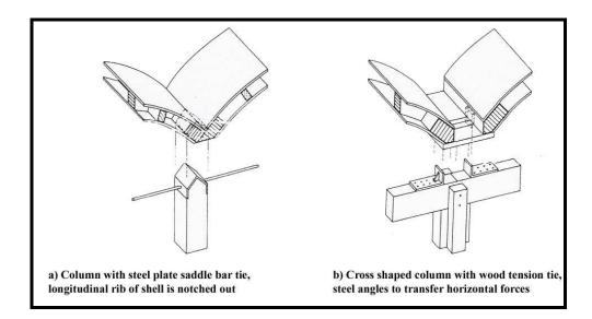
Figure II. 52 Column connection for hyperbolic paraboloid shells (Götz et al., 1989:167).
