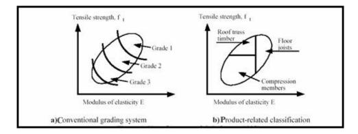
Figure II. 4 Mechanical properties of timber products required by end users (Kliger, 2000, document on-line).
