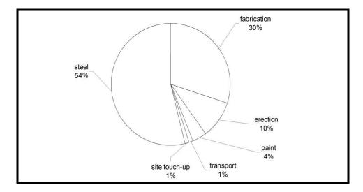
Figure III. 24 Cost breakdown of portal framed industrial steel structures (Owens 1992:913).
