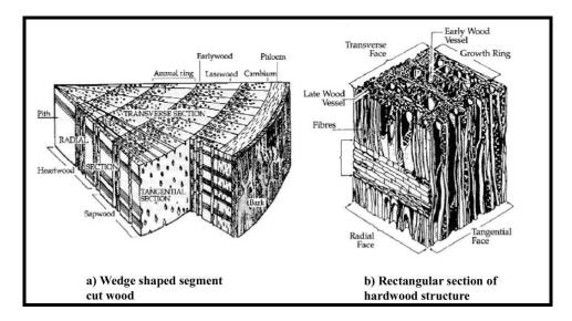
Figure A2. 2 Wedge-shaped segment cut from the bole of a hardwood and rectangular section of hardwood (Timber Research and Development Association, document on-line).
