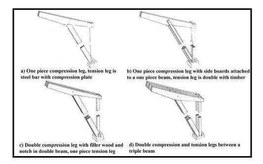
Figure II. 38 Frame leg details for two hinged frames (Götz et al., 1989:131).
