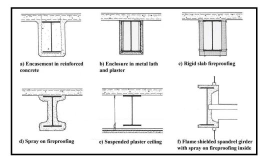
Figure III. 32 Some methods of fireproofing steel beams and girders (Allen, 1999:391).
