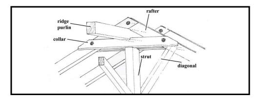
Figure II. 13 Ridge connection in a three purlin hip roof is composed of rafters, purlins, collars, struts and diagonals (Binan, 1990:82).
