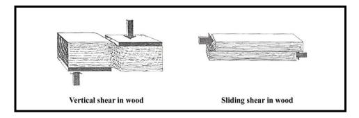
**Figure III. 7** Vertical shear in wood is a shearing that is perpendicular to the grain. Sliding shear in wood is a shearing stress that is parallel to the grain (Oberg, 1963:82).
