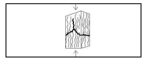
**Figure III. 5** Breakdown of a test specimen under a compressive load applied parallel to the grain (Karlsen, 1989: 22).
