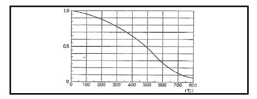
Figure III. 30 Reduction factor for steel's stifness at high temperatures (Eggen et al., 1995:36).
