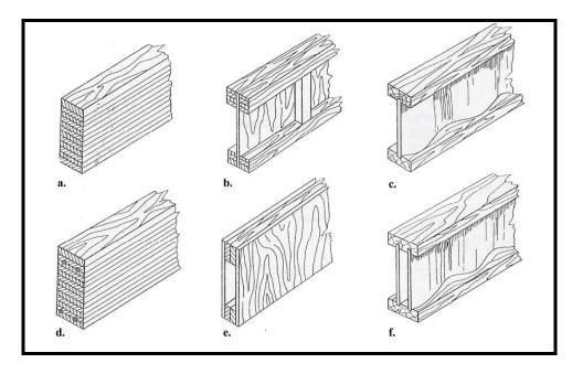
**Figure II. 3** Typical sections of glued laminated structures: a) solid rectangular section, b) 'I' section with a plywood web, c) 'I' section with a corrugated web, d) reinforced section, e) box shaped section, f) box shaped corrugated section (Karlsen, 1989:377).
