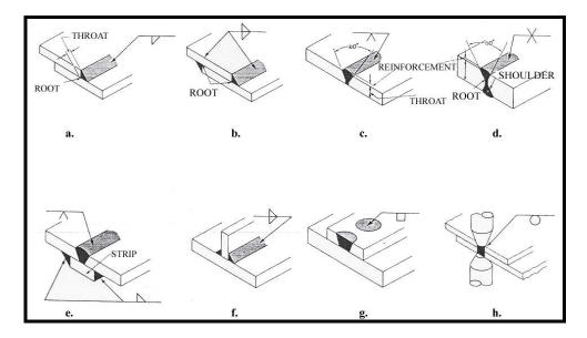
Figure III. 22 Types of welded joints: a) and b) Lap weld; c) and d) Groove weld; e) Single vee groove; f) Double fillet tee joint; g) Plug or rivet weld; h) Spot weld (Ellison, 1987:211).
