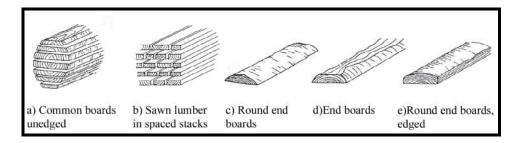
Figure II. 1 Five cutting ways of sawn lumber (Götz et al., 1989:21).
