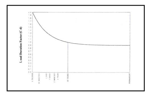
Figure III. 2 Duration of maximum load, load duration factors for various durations, decrease by the increasing time (Halperin, 1994:15).
