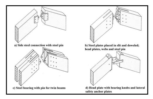
Figure II. 37 Crown hinge details for timber frames are composed of various arrangements (Götz *et al.*, 1989:119).
