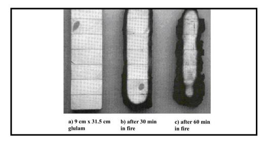
Figure III. 28 The effect of fire at 30 and 60 minutes on a glulam piece, dimensions of the beam is 9 cm by 31.5 cm before fire (Glued Laminated Timber Association, Technical Data Sheet, document on-line).
