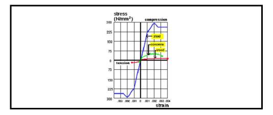
Figure III. 3 Stress strain diagram of steel and wood (Ocshorn, 1998, document on-line).
