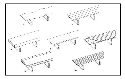
Figure II. 10 Roof decking arrangements are: a) Fabric or plastic roof on braced beams, b) Tongue or groove planking or splined boards, c) Composite materials, d) Wood chipboards, plywood or furniture panels, e) Diagonal planking, f) Panel elements of timber slats or sheating, g) Trapezoidal sheet metal (Götz *et al.*, 1989:127).
