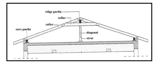
Figure II. 9 Structural members in a hip roof construction (Toydemir, 2004:40).
