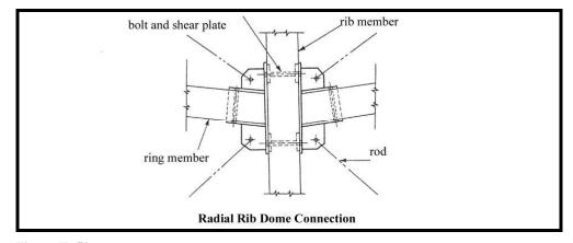
Figure II. 59 The connections of the rib members are critical. Radial rib dome connection is illustrated in the figure (Faherty, 1989: 9.46).
