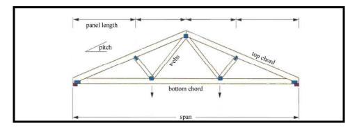
Figure II. 25 Typical truss members and definitions in truss design (MiTek Solutions, document online).
