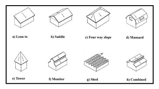
Figure II. 11 Classification of roof forms (Özdemir, 2003:90-91).
