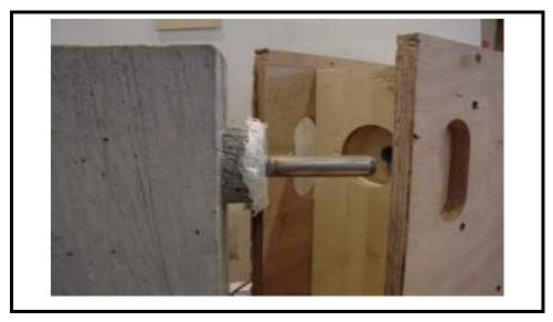
Figure III. 20 Timber with concrete connection is made with a 20 mm steel dowel (Kuilen, J-W.G., document on-line).
