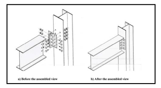
Figure III. 23 Exploded and assembled views of a framed, bolted beam to column flange connection, the size of the angles and the number of the bolts are decided by the magnitude of the load that the connection should transmit from beam to column (Allen, 1999:362).
