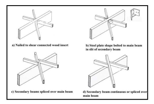
Figure II. 20 Secondary girders are placed on main girders in various alternatives with 60° (Götz *et al.*, 1989:107).
