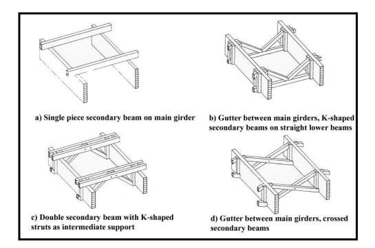
Figure II. 19 Secondary girders are placed on main girders in various alternatives with 90° (Götz *et al.*, 1989:109).
