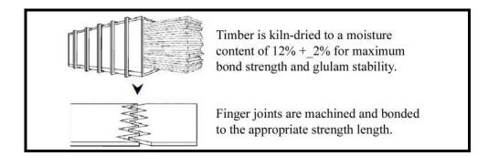
Figure II. 5 Production of glulam is composed of drying and jointing periods of laminates (Glued Laminated Timber Association, Glulam Specifiers Guide, document on-line).
