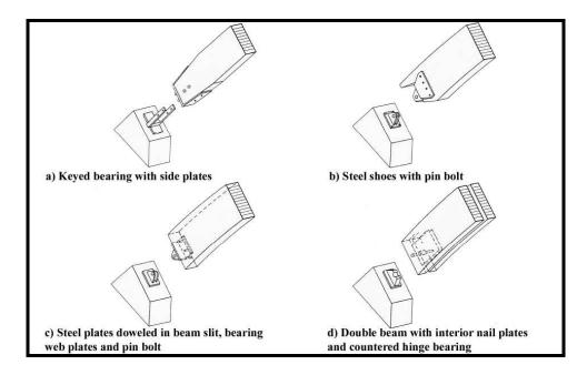
Figure II. 35 Base bearings of arches, the system can be also used in frames and beams (Götz *et al.*, 1989:147).
