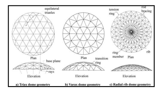
Figure II. 58 General dome geometry types: a) triax, b) varax, c) radial dome (Faherty, 1989:9.45, 9.47, 9.48).
