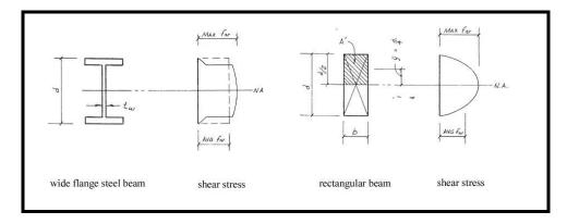
Figure III. 8 Horizontal shear stress distribution on a wide flange steel beam and rectangular wooden beam (Breyer, 1988:185).
