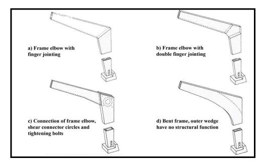
Figure II. 39 Frame leg details for three hinged frames (Götz *et al.*, 1989:133).
