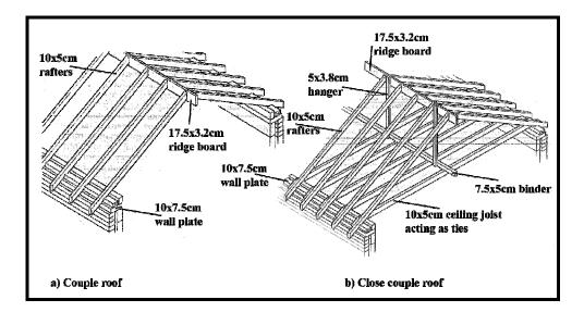
Figure II. 15 Ridge roofs are constructed in couple and close couple form (Foster, 1983:177).
