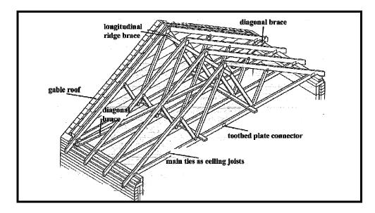
Figure II. 17 Trussed rafter roof construction (Foster, 1983:191).
