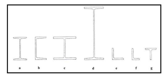
Figure II. 6 Typical hot rolled steel sections (Foster, 1983:143).
