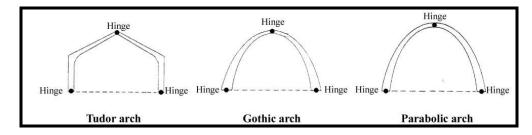
Figure II. 34 Three hinged arches have three general forms (Hornbostel and Hornung, 1982:183).
