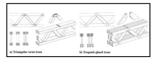
Figure II. 27 Triangular struts are glued by finger joints, in trigonit girder truss diagonals are joined by finger joints, double or triple flanges are nailed together with each nail loaded in double shear (Götz *et al.*, 1989:55-56).
