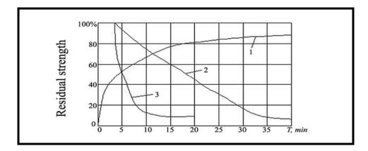
Figure III. 26 Strength vs fire temperature:1-standard curve for temperature variation during fire 2residual strength of a 5x10 cm wooden member 3-residual strength of a steel member (Karlsen, 1989:51).
