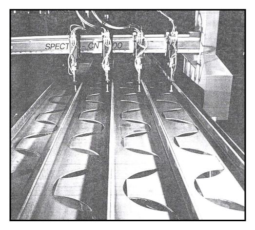
Figure II. 8 Production of castellated beams with the help of digital blow torches at Westok Structural Services Ltd., Wakfield, England (Eggen *et al.*, 1995:39).
