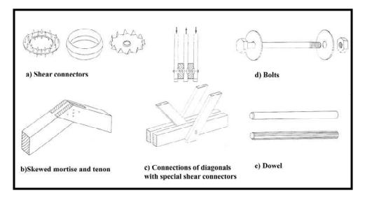
Figure III. 16 Typical timber connections used for jointing timber pieces (Götz et al., 1989:47).
