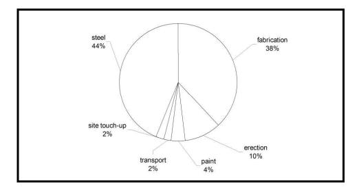
Figure III. 25 Cost breakdown of lattice steel structures in U.S.A. (Owens 1992:915).
