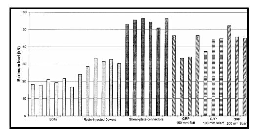
Figure III. 18 High performance jointing systems for timber. GRP: Glass Reinforced Plastic (Peter A. Claisseu, Tim J. Davis, 1998:415-425).
