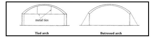
Figure II. 33 Two hinged arches are constructed in two ways (Hornbostel and Hornung, 1982:182).
