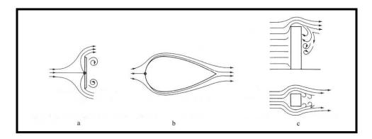
Figure III. 1 Wind flow about different shapes (Schodek, 1980:92).
