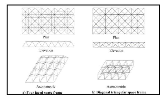
**Figure II. 44** Types of space frames: a) four faced, b) diagonal triangular (Toydemir *et al.*, 2004:138-139).
