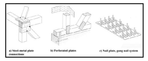
Figure III. 17 Various connections are used for jointing timber members (Götz et al., 1989:52).
