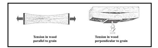
Figure III. 6 Tension in wood parallel and perpendicular to grain (Oberg, 1963:81).
