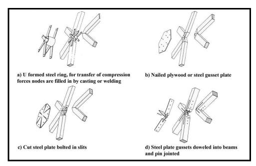
Figure II. 60 Various joint details in dome assembly (Götz et al., 1989:165).
