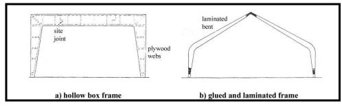
Figure II. 36 Frame structures are arranged two different ways (Foster, 1983:350).
