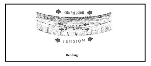
Figure III. 9 Bending a length of wood sets up multi-stresses: compression, shear and tension (Oberg, 1963:83).
