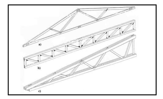
**Figure II. 28** a) Nail plate truss: Node plates consist of galvanized steel plates, they are pressed from both sides into wood. b) Greim truss: Stell plates are placed in sawn mortises and nailed from the outside without predrelling. c) Menig truss: Node plates are placed between struts and are not visible in the finished truss (Götz *et al.*, 1989:58).
