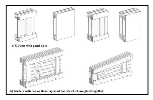
Figure II. 18 Girders are composed of 'I' or box sections with panels or with glued boards (Götz *et al.*, 1989:57).
