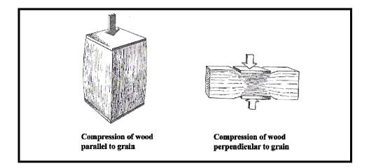
Figure III. 4 Compression of wood parallel and perpendicular to grain (Oberg, 1963:80).
