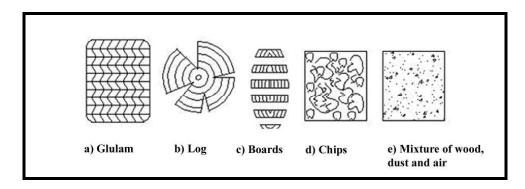
Figure III. 27 Fire resistance of various wood members and materials. Glulam and log are the most fire resistant, in boards and chips fire resistance decrease, the mixture of wood dust and air is regarded as explosive (Karlsen, 1989:51).
