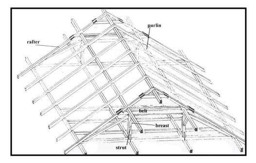
Figure II. 14 Two purlin hung roof is composed of rafters, purlins, diagonals, collars and struts (Binan, 1990:94).
