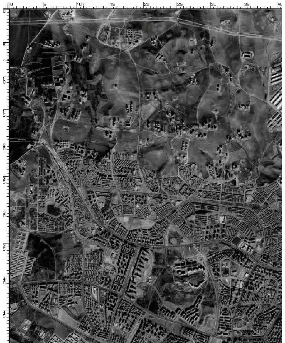
Figure 4.2: Single band, grayscale Image (SPOT Pan) of size (4800 x 3600) with spatial resolution 10m.
