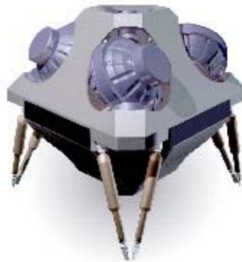
Figure 3.3 CMGs installed on a ground test bed ( from [16])
