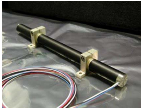
Figure 3.5 A typical magnetic torque rod (from [29])
