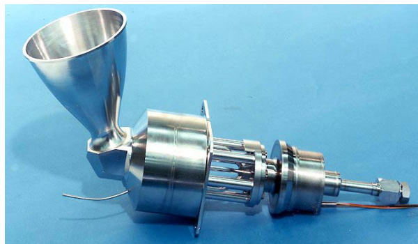
Figure 3.4 A thruster for use in space applications (from [11])
