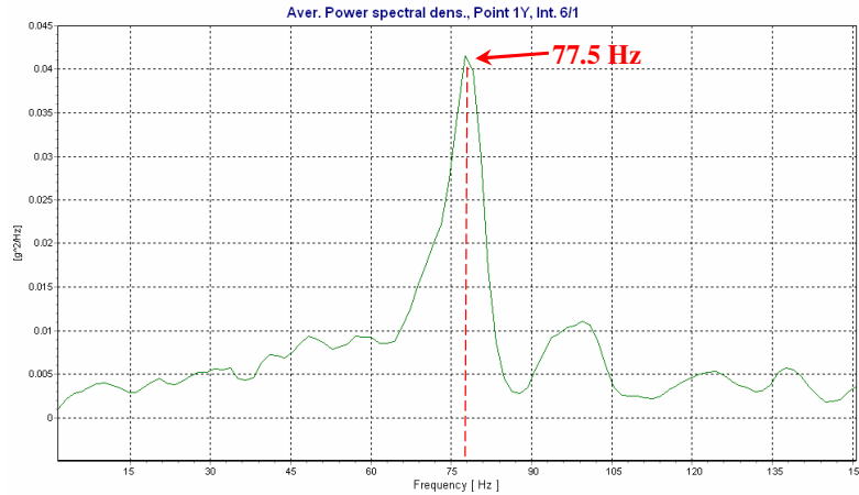
Figure 6.16: PSD graph of the accelerometer on the cowling in transverse axis.
