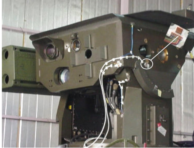
Figure H.1: Strain gage application on a missile launcher system [7].
