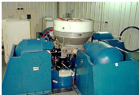
Figure 4.1: An example of multiaxial vibration test equipment.
