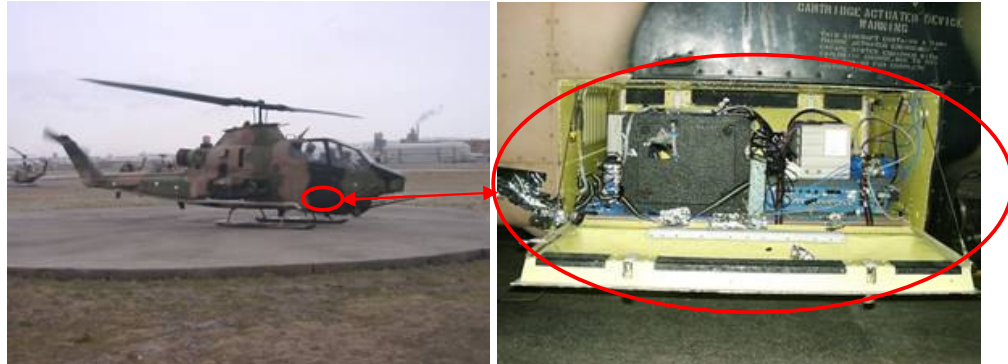
Figure 5.5: Location of the data acquisition system during the flight tests.
