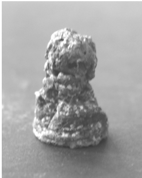
Figure 4.8. Photograph of a collapsed foam. (Al-8% Al 2 O 3 -fineTiH 2 , 805°C) (Diameter: 15 mm)
