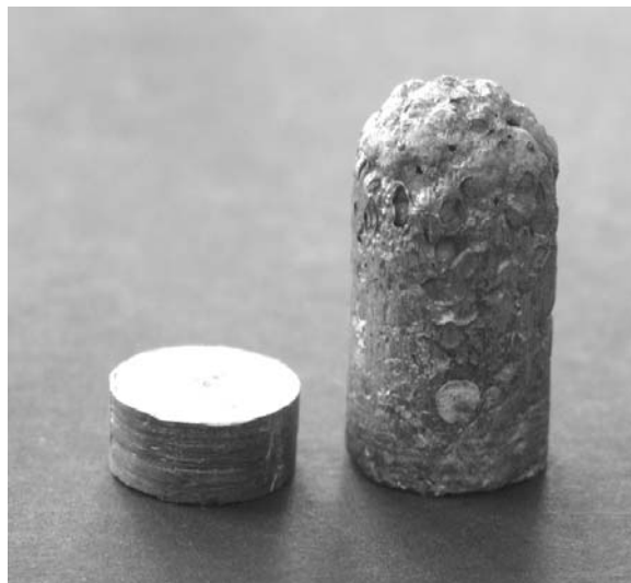
Figure 4.4. Photograph of a sample before and after foaming. (Al-8% Al 2 O 3 -coarse TiH 2 ) The samples are 15 mm in diameter.
