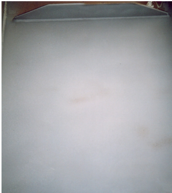
Figure 30: Steel Panel Blasted with FS
