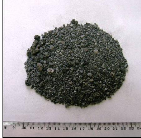
Figure 8: Coal Furnace Slag Sample
