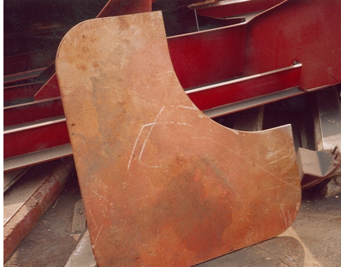
Figure 17: First Steel Plate before Blasting
