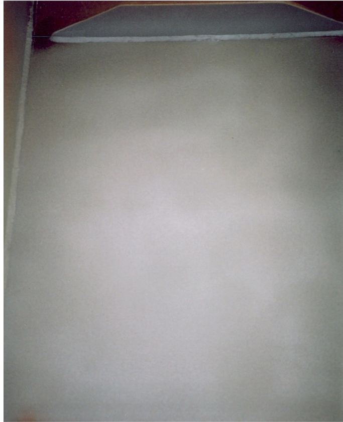
Figure 21: Steel Panel Blasted with CS
