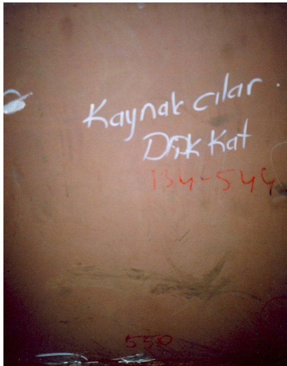
Figure 20: Steel Panel before Blasting
