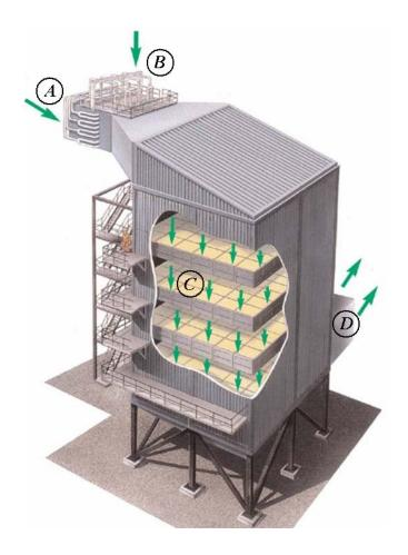
**Figure 1.1. A simple SCR reactor, A)** Flue gas containing  $NO_x$  is admitted from the boiler to the SCR reactor, **B**) Ammonia is added to the flue gas, **C**) The gas mixture flows over catalyst elements, which cause nitrogen oxides and ammonia to react, **D**) The reaction converts the nitrogen oxide to pure nitrogen and water (Figure is taken from the ABB Alstom Power Environmental Systems Brochure).
