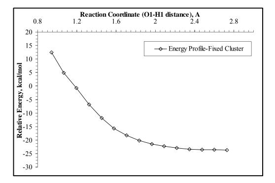
**Figure 4.42.** Energy profile for ammonia dissociation on fixed (001)  $Ti_2O_9H_{10}$  cluster.
