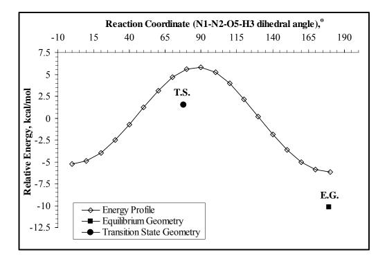
**Figure 4.15.** Energy profile for the isomerization reaction of the cis-HN=NOH species to form cis-HN=NO-trans-H species.
