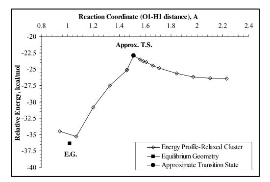
**Figure 4.43.** Energy profile for ammonia dissociation on relaxed (001)  $Ti_2O_9H_{10}$  cluster.
