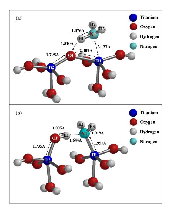
**Figure 4.44.** (a) Approximate transition state and (b) Equilibrium geometry of dissociated ammonia on relaxed (001)  $Ti_2O_9H_{10}$  cluster.
