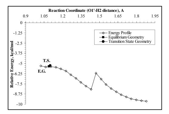
**Figure 4.13.** Energy profile obtained for the interaction of trans H-N=NOH species with the oxygen site (O1') of the cluster to form cis-HN=NOH species.
