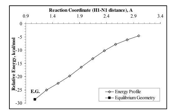
Figure 4.1. Energy profile for the Brønsted acidic ammonia activation.
