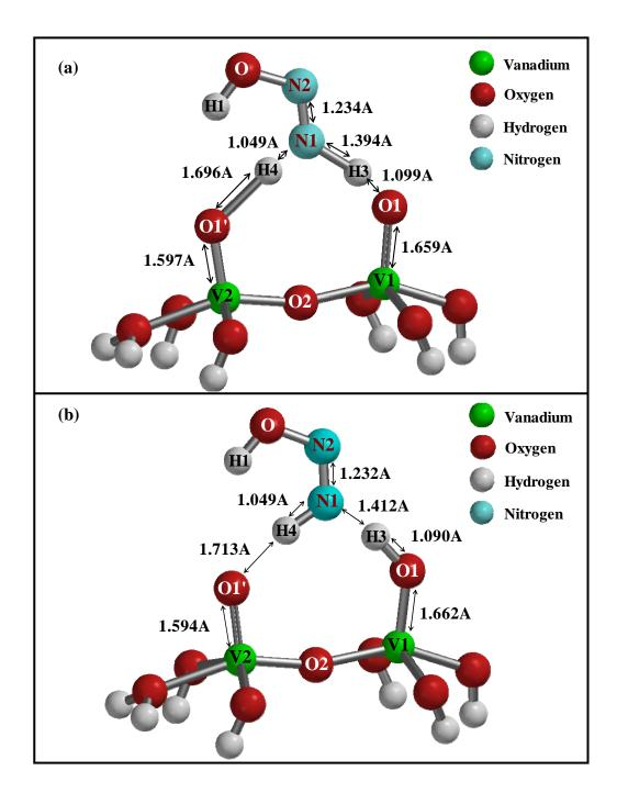
**Figure 4.14.** (a) Transition state geometry for the reaction of formation of cis-HN=NOH species from trans H-N=NOH species, (b) Equilibrium geometry of the adsorbed cis-HN=NOH species.
