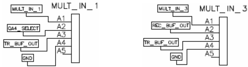
Figure 3.15: Signal selection pin connector blocks. MULT_IN_1 multiplexes one of the three available signals to the X1 input of the AD633 multiplier. MULT_IN_3 multiplexes one of the three available signals to the X2 input of the AD633 multiplier. X1 and X2 are 1 st and the 3 rd pins of AD633, respectively.
