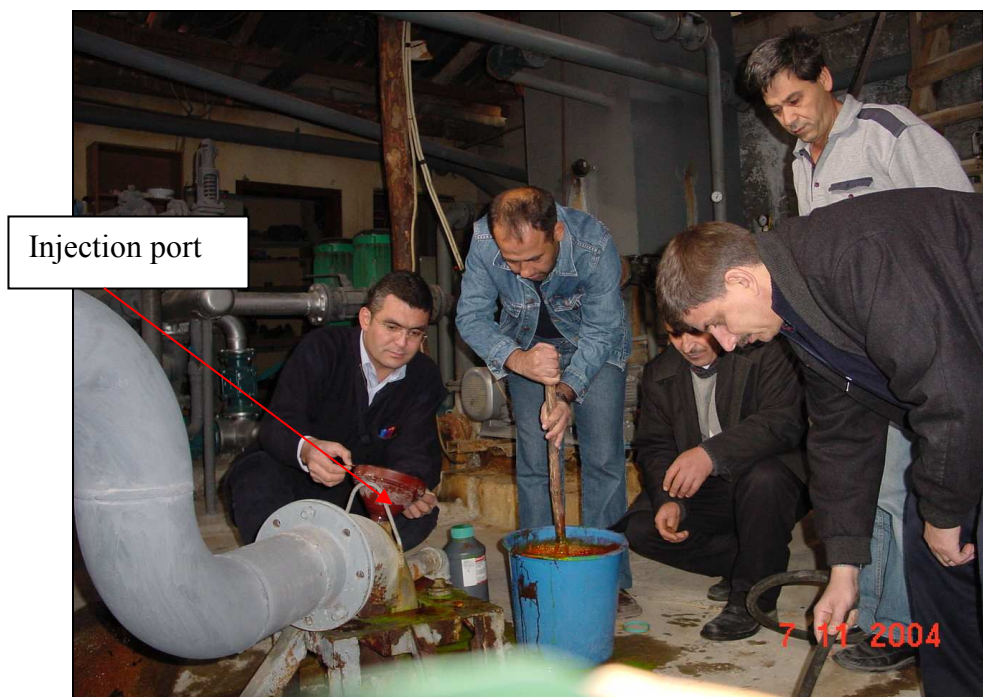
Figure 7.5 Tracer (Fluorescein) injection to MTA-1 well
