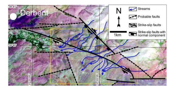
Figure 4.3 The displaced streams along the SFZ in around Derbent overlaid on ASTER image. Band combinations RGB:5,2,1 with saturation enhancement. Yellow box indicates the position of Figure 4.8.
