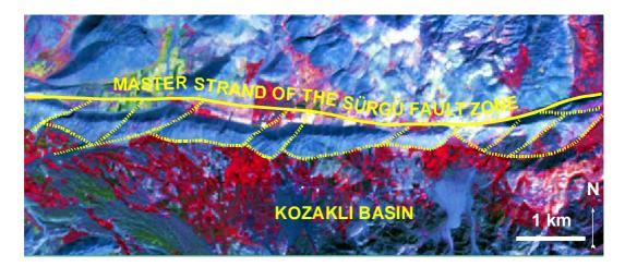
Figure 4.1 ASTER image (band combination; R:3, G:2, B:1) showing pressure ridges within an anastomozing en echelon pattern of faults (yellow lines).
