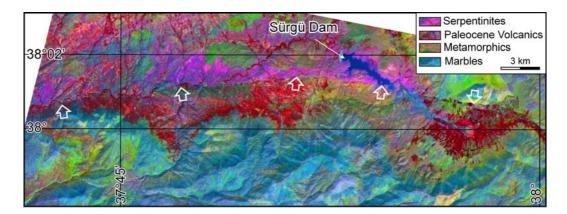
Figure 4.4 Trace Master Strand of the SFZ near Sürgü Dam indicated with white arrows and overlaid on Decorrelation stretched ASTER image. Band combinations; RGB:4,2,1. Note very sharp trace of the Master Strand of the SFZ.
