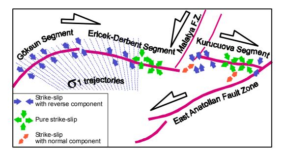
Figure 7.1 Simplified map showing the segments of the SFZ and orientation of horizontal components of constructed palaeostress configurations. Note 1) rotation of major principal stress as the trend of the fault changes (trajectories), 2) domination of strike-slip component over dip-slip from W to E and 3) domination of NE-SW extension in the east, S of Kurucova Segment, 4) position of Malatya Fault Zone.
