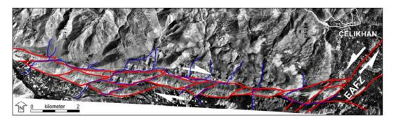
Figure 4.7 Aerial photo showing pressure ridges within an anastomozing en echelon pattern of faults (red) and dextrally displaced stream courses (blue). EAFZ: East Anatolian Fault Zone. Note that all the streams flow southwards.
