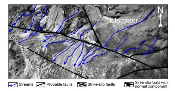
Figure 4.8 Deflected streams in E of Derbent and NW of Nurhak overlaid on the aerial photo. (See Figure 4.3 for its location)
