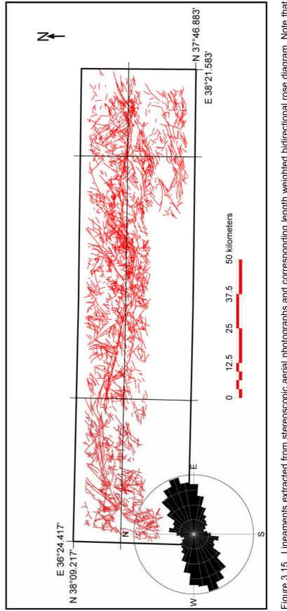
Figure 3.15 Lineaments extracted from stereoscopic aerial photographs and corresponding length weighted bidirectional rose diagram. Note that ENE-WSW lineaments are dominated and Malatya Fault trend (N10°-20°E directions) is also expressed. (see Appendix-A for a larger view of this figure)
