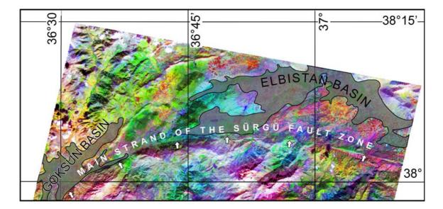
Figure 4.6 Subset of an ASTER image depicting a very sharp trace of the SFZ (for the sake of clarity fault trace is not delineated but indicated with arrows). The image is produced by DS and PCA. Band combination; RGBI:5,3,1, intensity is PC-1.
