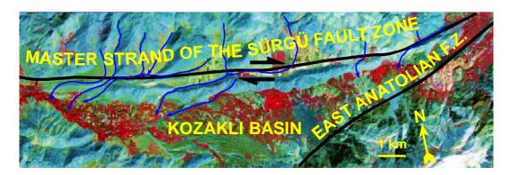
Figure 4.2 ASTER image (band combination; R:3, G:2, B:1) showing dextrally displaced streams along the SFZ between Çelikhan and Sürgü
