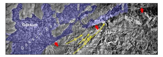
Figure 4.9 Aerial photo showing western part of the study area. Main Strand of the SFZ is dipping northwards and is indicated with red arrows. Singly plunging anticlines and synclines are indicated with yellow lines.
