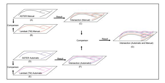
Figure 3.16 Process flow of the final lineament map for the study area.
