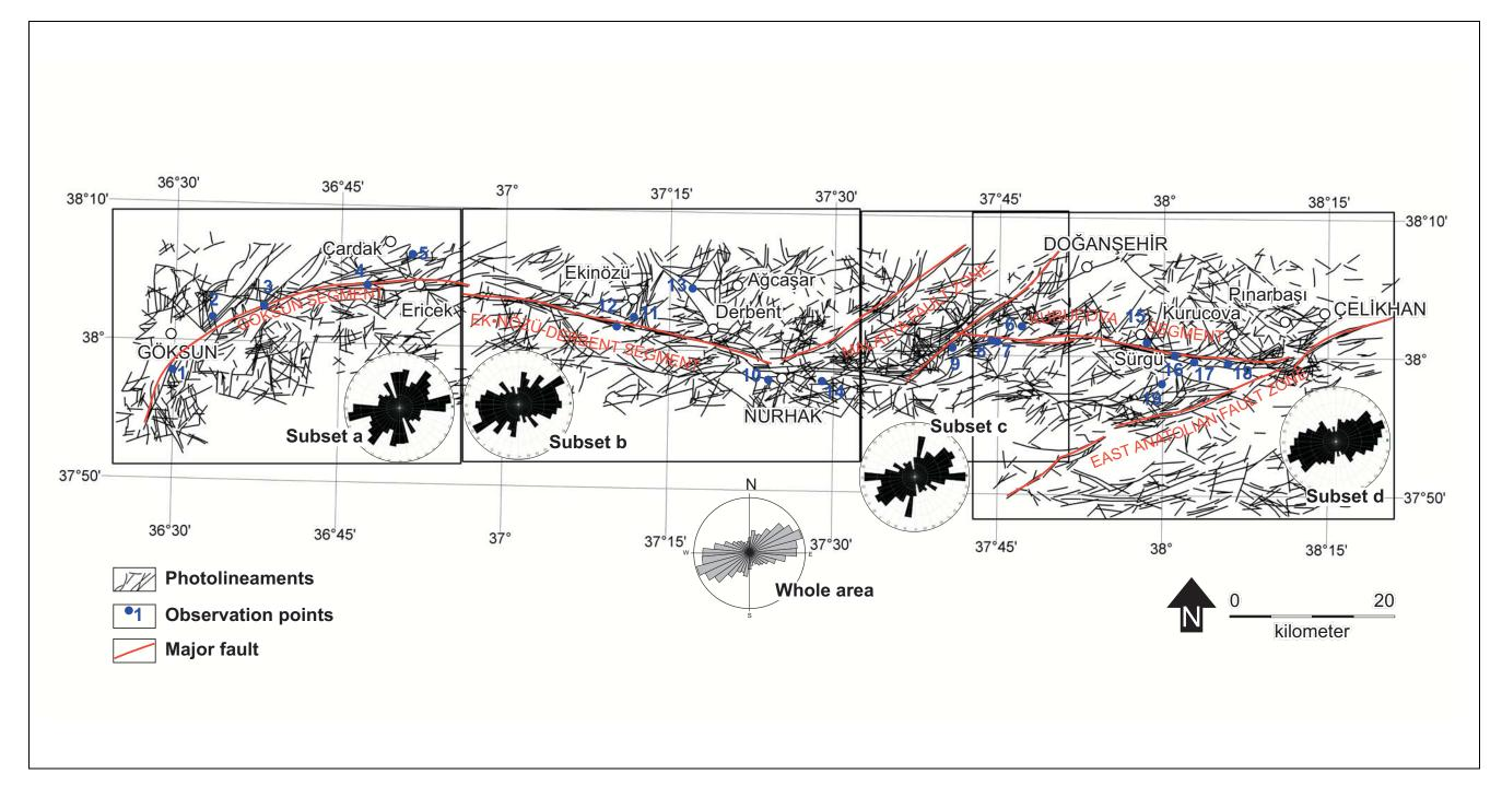
Figure A.1 Local lineament map of the Sürgü Fault Zone extracted from the aerial photographs.
