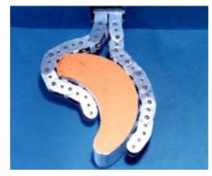
Figure (2.22-b) The flexible gripping action of the Soft Gripper I Figure (2.22) Hirose's Soft Gripper I
