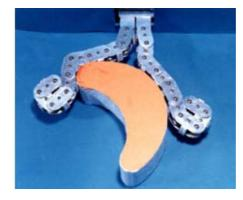
Figure (2.22-a) The flexible gripping action of the Soft Gripper I
