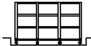
Figure 2.12. 2-D Simple Model of A Building with Base Isolation
