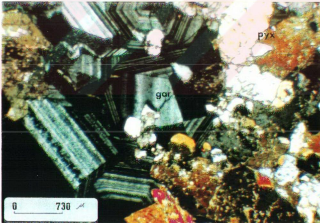
Figure 6.11. Photomicrograph displaying euhedral to subhedral garnets (gar) that show oscillatory zoning (pyx: pyroxene)
