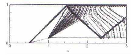
Figure 7.3f Comparison of Mach Number Contours for Wedge at  $M_{\infty} = 2$
