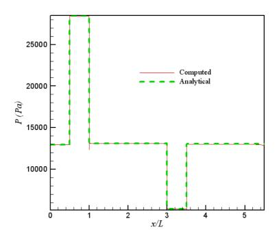
Figure 7.1f Computed and Analytical Pressure Distributions at  $M_{\infty} = 2$
