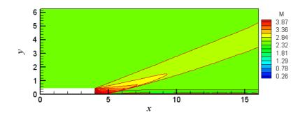
Figure 7.2c Mach Number Contours for Backward-Facing Step at  $M_{\infty} = 2.5$
