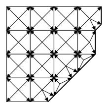
Figure 6.1 Reconstruction to Find Nodal Values from Cell-Centered Ones
