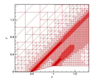
Figure 7.1a Final Mesh around the Forward-Facing Ramp at  $M_\infty=2$
