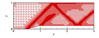
Figure 7.3a Final Mesh for Wedge at  $M_{\infty} = 2$
