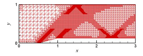
Figure 4.9a Mesh after 3 Levels of Solution Adaptation
