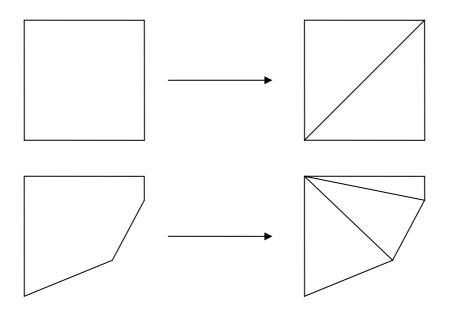
Figure 6.2 Cell Triangulation
