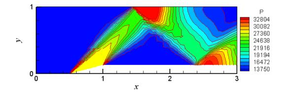
Figure 4.7b Pressure Contours after 1 Level of Solution Adaptation
