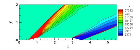
Figure 7.1d Pressure Contours at  $M_{\infty} = 2$
