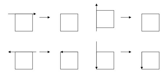
Figure 3.4 The Modification to the Original Liang-Barsky Algorithm
