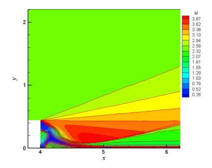
Figure 7.2e Mach Number Contours around the Step at  $M_{\infty} = 2.5$
