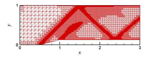
Figure 4.10a Mesh after 4 Levels of Solution Adaptation
