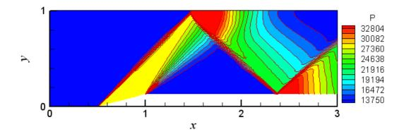
Figure 4.9b Pressure Contours after 3 Levels of Solution Adaptation
