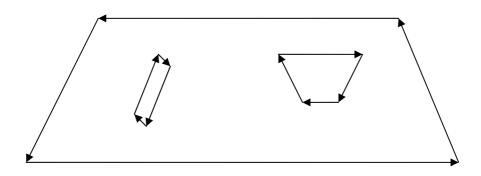
Figure 3.11 Oriented Boundaries Representing a Simple Closed Region
