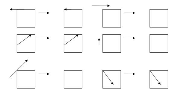
Figure 3.5 Special Cases of Line Segment-Rectangular Region Interactions
