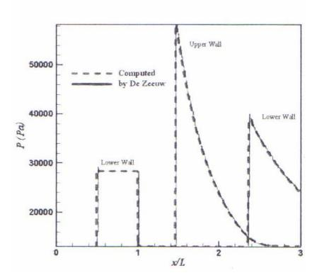
Figure 7.3e Comparison of Pressure Distributions for Wedge at  $M_{\infty} = 2$
