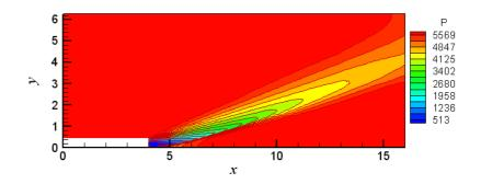
Figure 7.2b Pressure Contours for Backward-Facing Step at  $M_{\infty} = 2.5$
