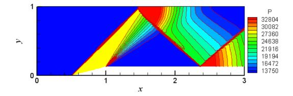
Figure 4.10b Pressure Contours after 4 Levels of Solution Adaptation
