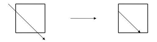
Figure 3.2 Clipping of an Oriented Line Segment against a Rectangular Region
