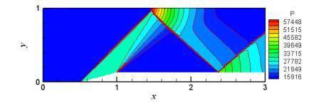
Figure 7.3c Pressure Contours for Wedge at  $M_{\infty} = 2$
