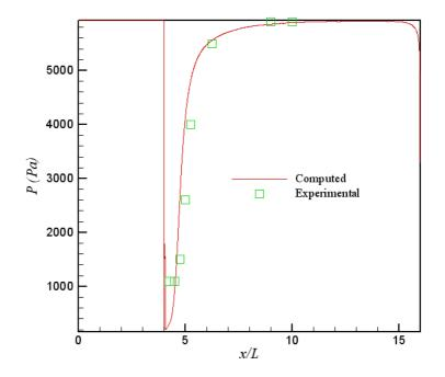
Figure 7.2f Computed and Experimental Pressure Distributions
