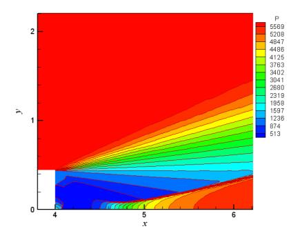
Figure 7.2d Pressure Contours around the Step at  $M_{\infty} = 2.5$
