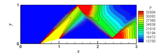
Figure 4.8b Pressure Contours after 2 Levels of Solution Adaptation
