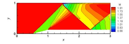
Figure 7.3d Mach Number Contours for Wedge at  $M_{\infty} = 2$
