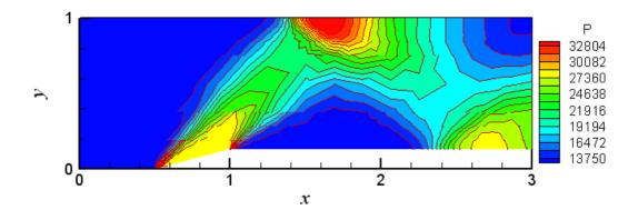
Figure 4.6b Pressure Contours without Any Solution Adaptation
