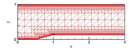
Figure 4.6a Mesh without Any Solution Adaptation
