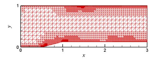
Figure 4.7a Mesh after 1 Level of Solution Adaptation
