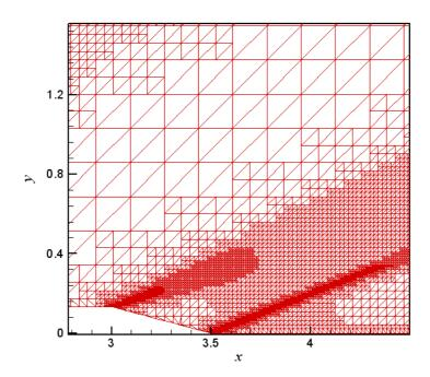
Figure 7.1b Final Mesh around the Backward-Facing Ramp at  $M_\infty=2$
