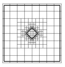
Figure 4.4 Cut-Cell Adaptation
