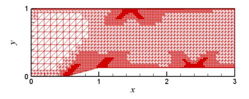
Figure 4.8a Mesh after 2 Levels of Solution Adaptation
