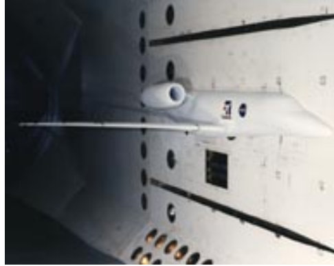
Figure 3. 3: A Cessna Aircraft, modeled and instrumented for aeroelastic experiments at TDT
