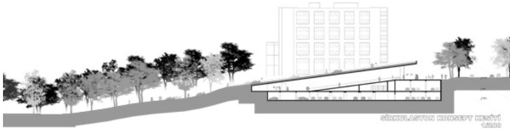
Figure 19 Section demonstrating the suggestion of S. Erdem and G. Erdem about lower and upper level ground relationships and evaluating the vista potential of the area by grass ramp.
