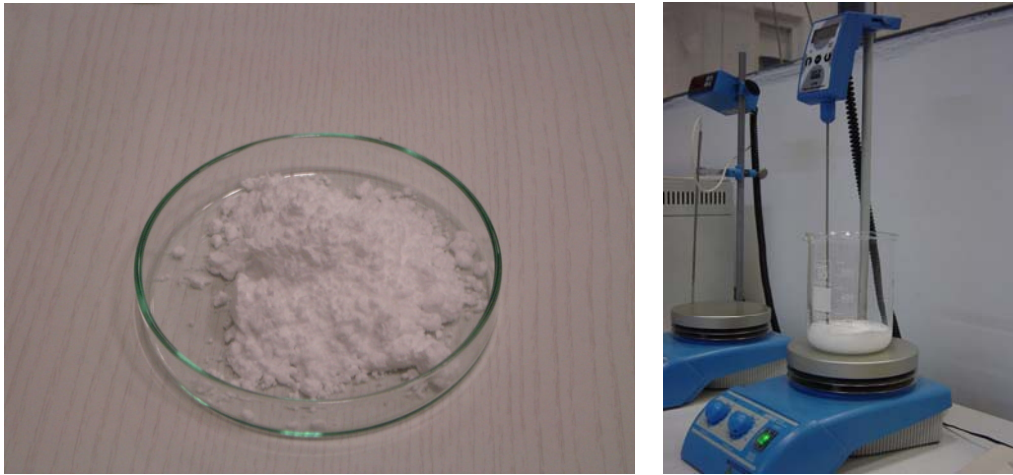
Figure 3.1.2. (a) The surfactant hexadecyltrimethylammonium bromide ( C_{16}H_{33}(CH_3)_3NBr ) (b) Starting to stir surfactant solution
