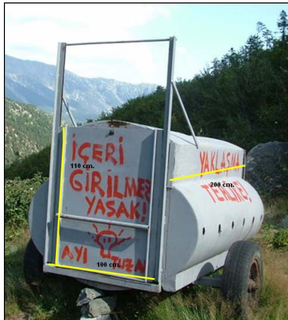
Figure 2.5 Modified culvert trap for brown bears
