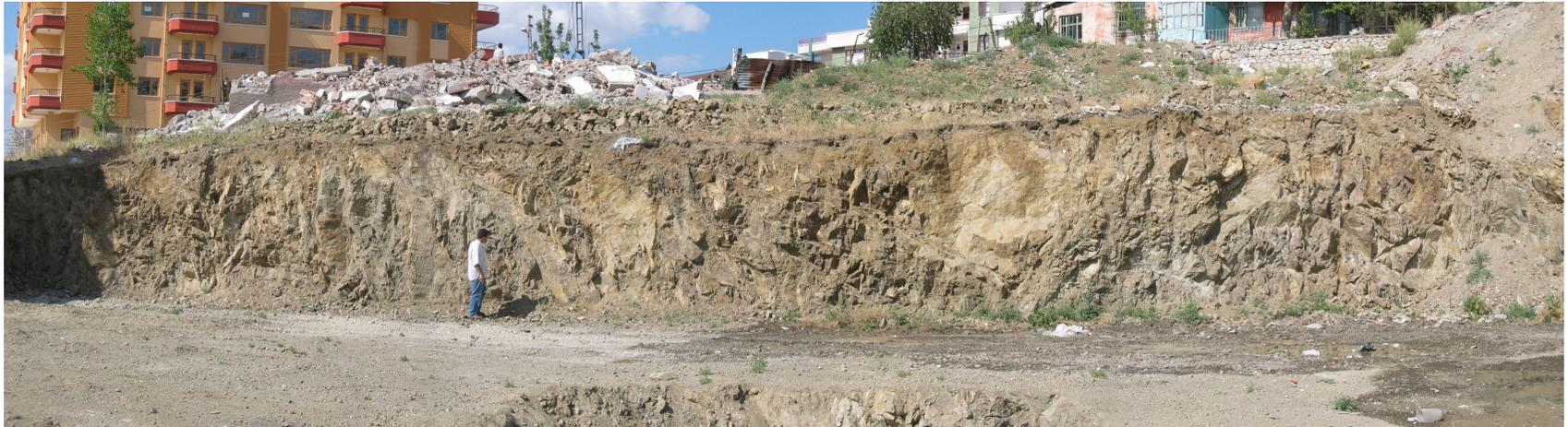
Figure 4.5 General view of the greywacke rock mass from a foundation cut near the boreholes 1 and 2 at CAKS.
