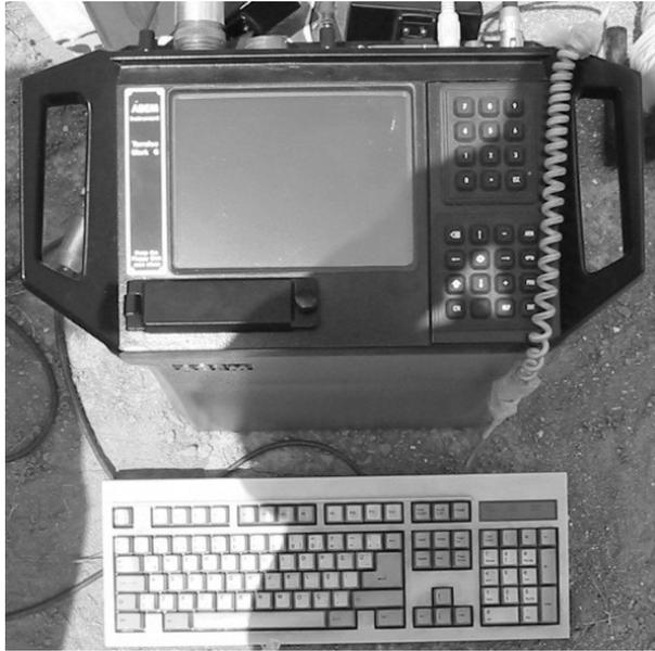
Figure 4.27 The seismometer used during the seismic refraction surveys.
