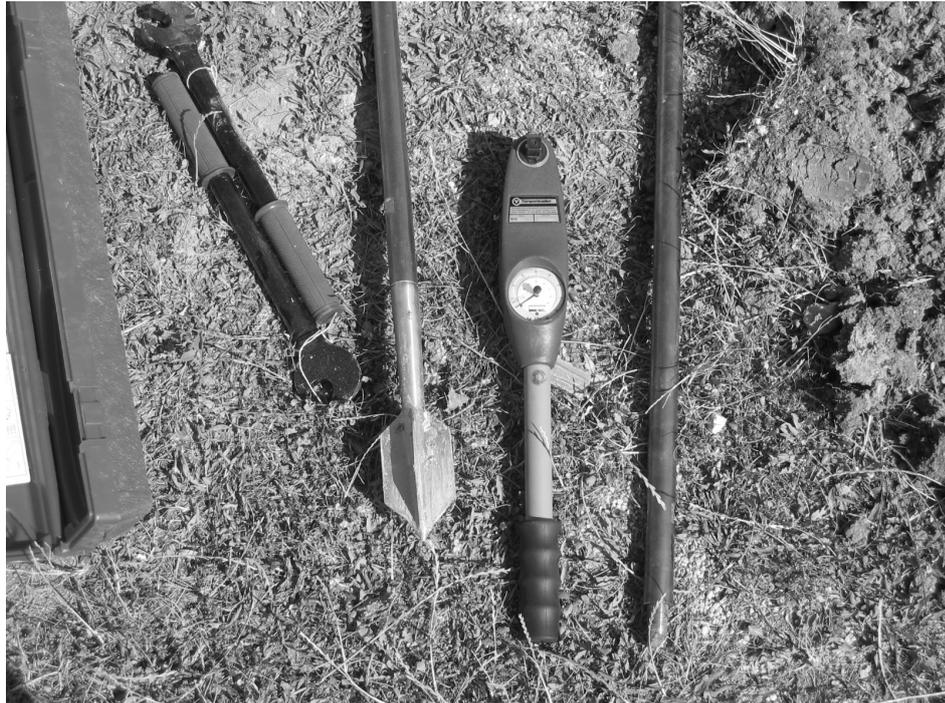
Figure 4.32 Field vane used in the study.
