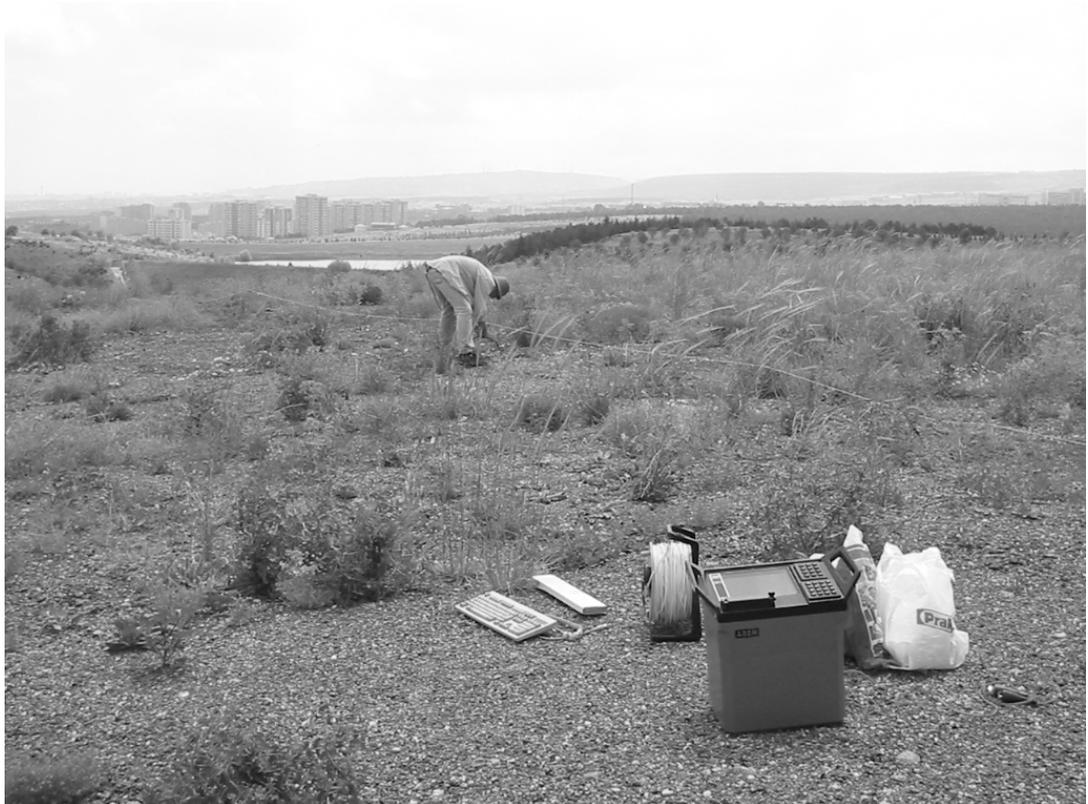
Figure 4.28 Field layout of the refraction survey at Beytepe campus of Hacettepe University, Beyaz Ev location.
