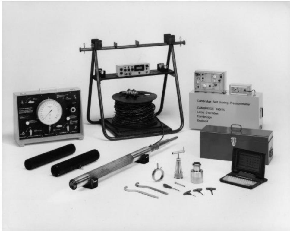
Figure 4.11 Self boring pressuremeter kit probe and control parts (Cambridge In-situ, 2005).
