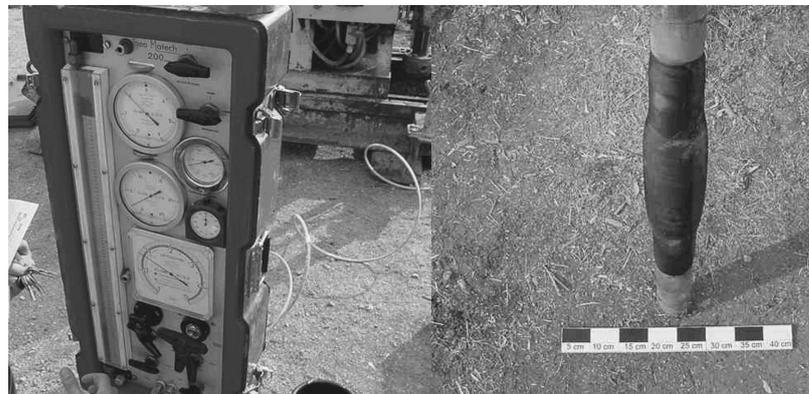
Figure 4.8 Ménard Pressuremeter (type GC) and its probe used in this study.
