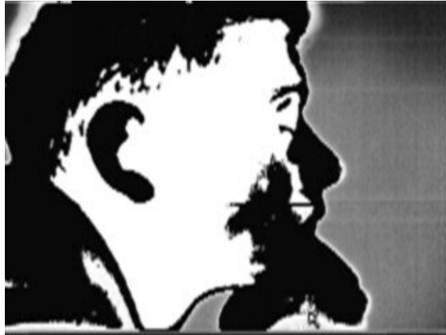
Figure 3-8 Output of the Laplacian Filter Showing the Edges at the Input Image
