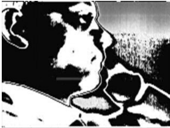
Figure 3-14 Output Image After the Prewitt Filter Showing the Edges at the Input Image
