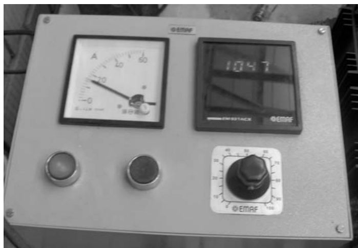
Figure 4.4 Control Panel of the Wind Tunnel
