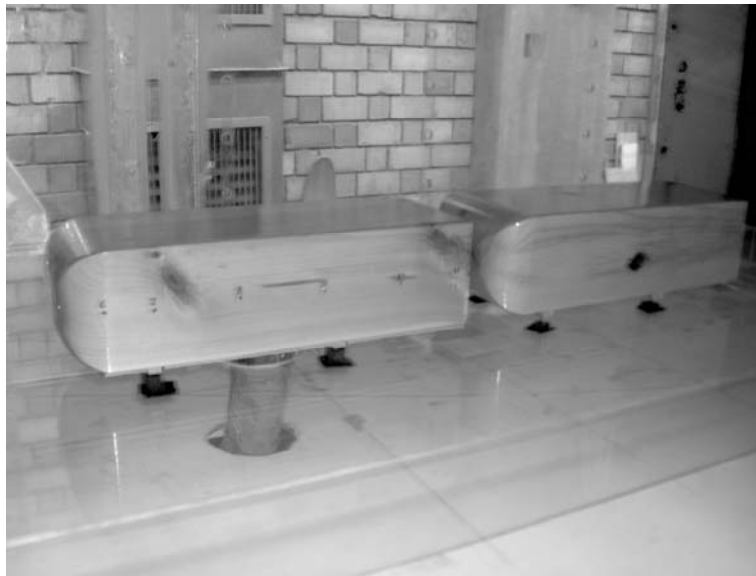
Figure 5.18 Surface Pressure Measurement for the Ahmed Body in Close-following Situation
