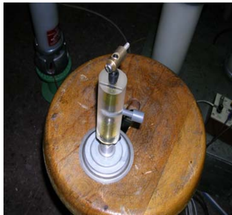
Figure 4-10 Internal Discharge Electrode Sample with a cavity
