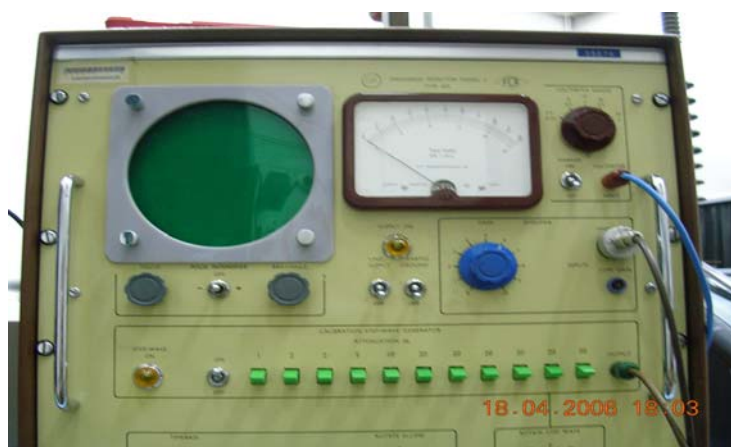
Figure 4-1 ERA Discharge Detector
