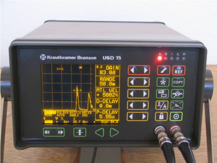
Figure 4.5 Krautkramer Branson USD 15 digital oscillator
