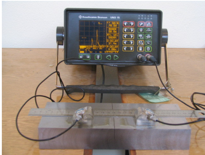
Figure 4.7 The TOFD Method test setup
