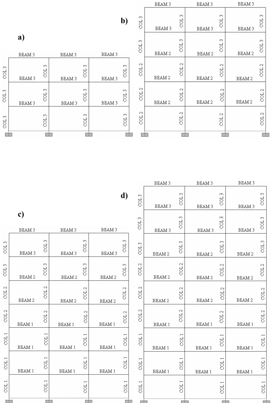
Figure 3.3a) 3 story model, b) 5 story model, c) 7 story model, d) 9 story model.
