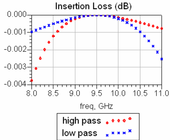
Figure 3.13 Insertion Losses of the two states of the ideal 90° HP/LP phase shifter
