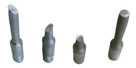
Figure 4.8 Macroscopic fracture surfaces Cup and cone structure indicates the ductile fracture behavior
