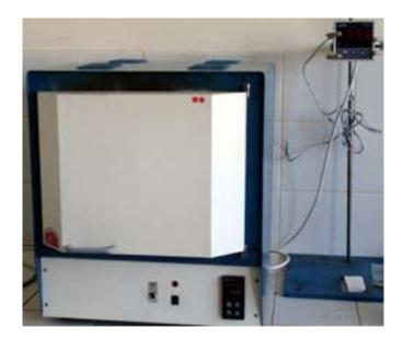
Figure 3.2 Muffle furnace for solutionizing
