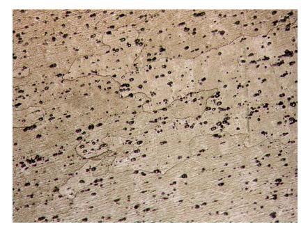
Figure 4.1 Microstructure of as-received Al 6066 (200X) Dark phases present throughout the surface
