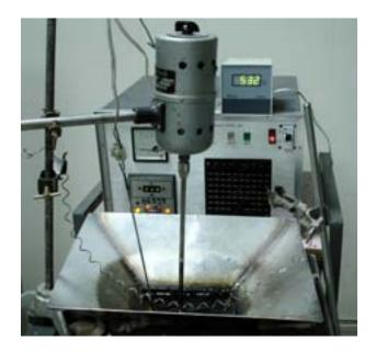
Figure 3.3 Salt bath for solutionizing
