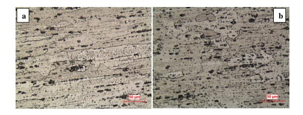
Figure 4.18 Sample treated at 450°C for 1 hr after 40% cold deformation (LD) a)center b)near rim
