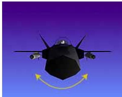
Roll (wings roll up or down)
