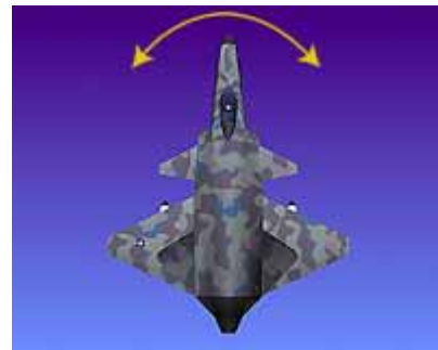
Yaw (nose moves from side to side)
