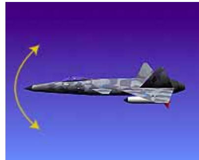
Pitch (nose pitches up or down)
