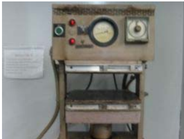
Figure 3.3 Schematic representation of hot-press machine used in this work
