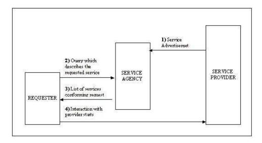
Figure 2. 3 Interaction between parties involved in the usage of a Web service
