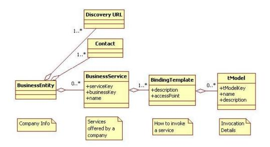
Figure 2. 7 UML representation of UDDI data elements
