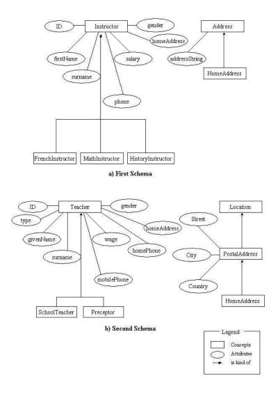
Figure 3. 2 Examples of heterogeneities between schemas
