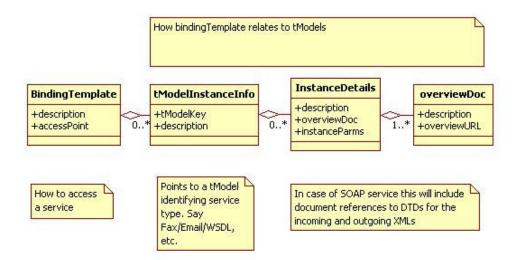
Figure 2. 8 Relationship between bindingTemplates and tModels
