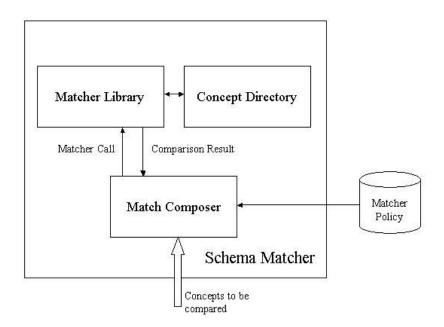
Figure 4.9 Schema Matcher architecture
