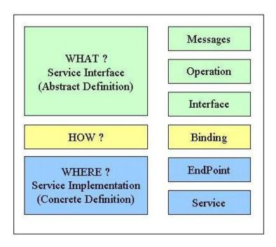
Figure 2.4 Conceptual view of WSDL Component Model
