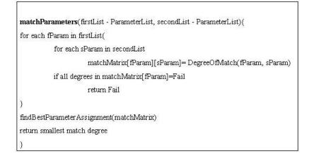
Figure 4.7 Algorithm for matching parameters
