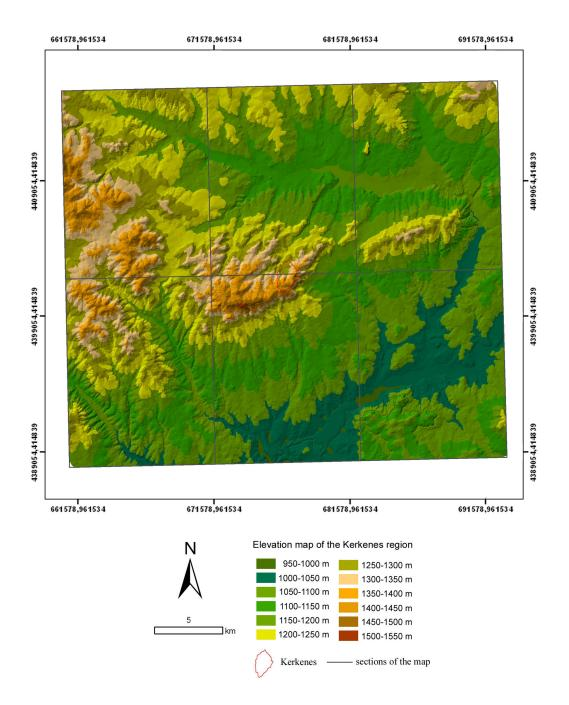
Figure 3.2. Elevation map of the Kerkenes region produced from six sheets of 1:25000 topographic maps as a TIN Model.
