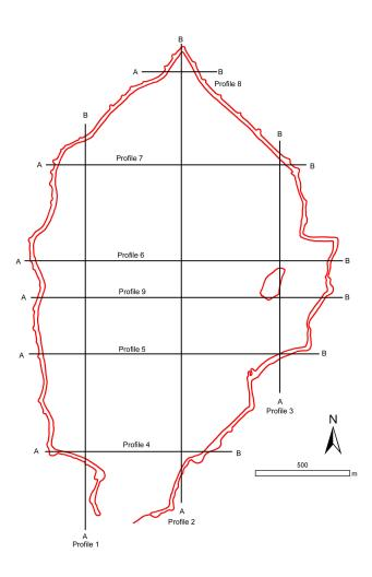
Figure 3.13. Sample terrain profiles for Kerkenes (Profiles 1-8 are every 500 meters and Profile 9 is randomly selected to show the terrain profile for the Kale)
