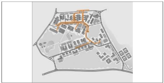
Figure- 4.35: Natural Gas System (Source: Archive of Teknopark Inc.)
