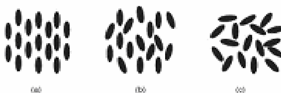
Fig. 1.1 The schematics of (a) crystal, (b) liquid crystal and (c) liquid state
