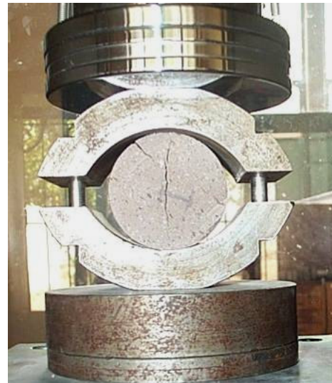
Figure 5. 5 Brazilian test specimen after test
