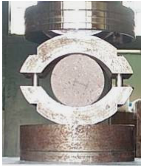
Figure 5. 4 Brazilian test specimen before test
