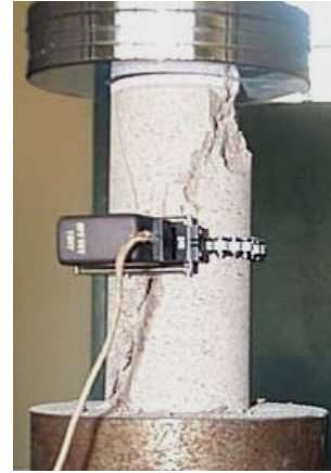
Figure 5. 2 UCS test specimen with circumferential extensometer after test
