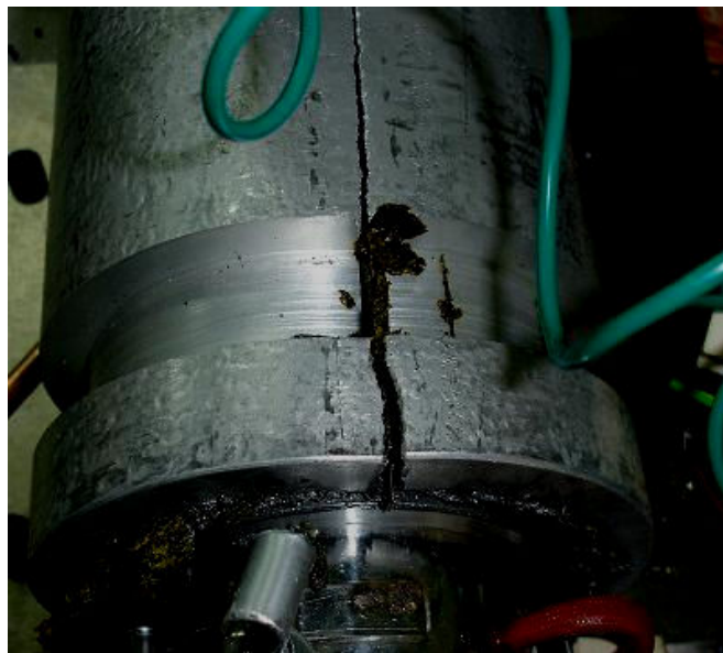
Figure 5.10: View of the failure on the vessel
