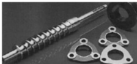
Figure 3.12: A view of barrel rings, screw shaft and bearing parts of the Mini 40 screw press manufactured by Rosedowns [37]
