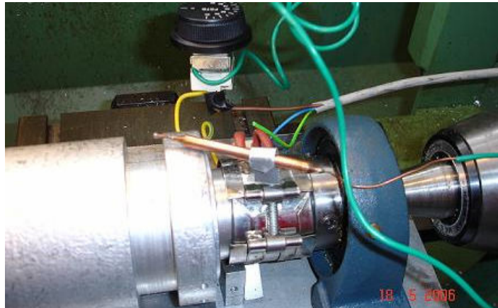
Figure 5.6: Heating Device mounted onto the third prototype
