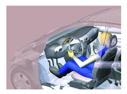
Figure 3.2 A typical posture adopted in the driving environment of a car (RAMSIS)
