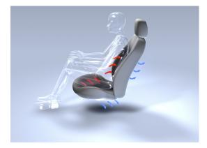
Figure 3.6 The effect of ventilating fans integrated in to the seat cushion and back Ref.<u>http://www.johnsoncontrolspress.com/ALL\_PressImages/passiveclimate\_100k.jpg</u> (03.10.2006)
