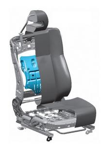
Figure 3.4 Contour and lumbar support development in the cad environment
