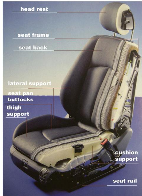
Figure 3.7 Cross-section of an advanced seat structure and components
