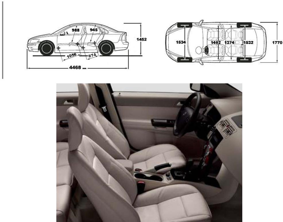
Figure 5.3 The Volvo S40 automobile dimensions (mm) and interior appearance
