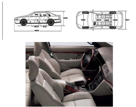
Figure 5.5 The Volvo S80 automobile dimensions (mm) and interior appearance
