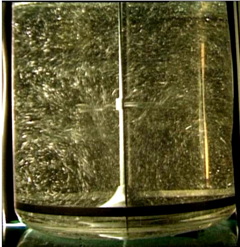
Figure 6.28 Lightsheet photo of mixer combination (1.5d)
