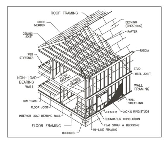
Figure 1.5 Overall view of residential steel framing and the basic components, NASFA Publication NT600
