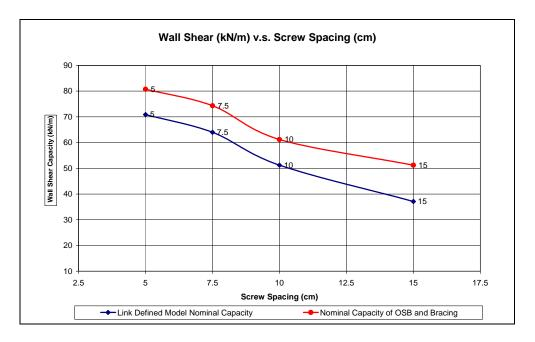
Figure 6.3 Nominal Capacities of Walls vs. Screw Spacing with and without Xbracing
