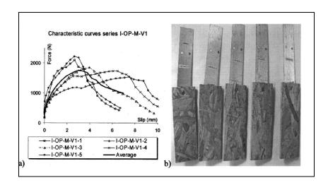
Figure 2.3 Experimental curves and failure modes of OSB to steel connections by Fülop and Dubina (2006)
