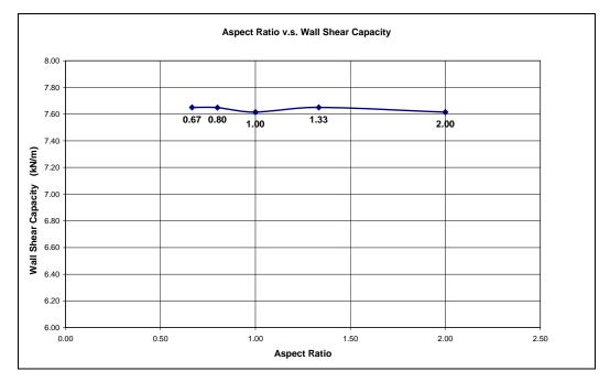
Figure 5.9 Change of Unit Wall Shear Capacity with Aspect Ratio curve
