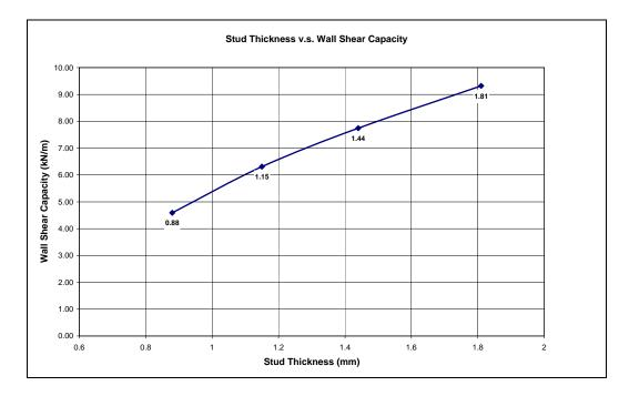
Figure 5.7 Stud Thickness vs. Wall Shear Capacity curve
