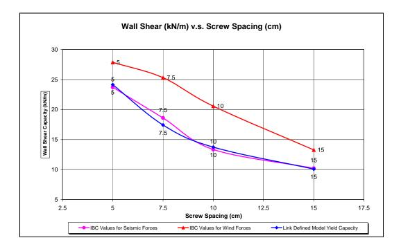
Figure 4.10 Comparison of Nonlinear Link defined Model yield Capacity with IBC nominal shear values for wind and seismic forces
