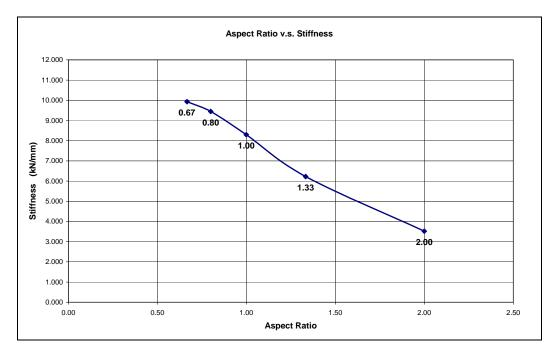
Figure 5.10 Change of Stiffness with Aspect Ratio curve
