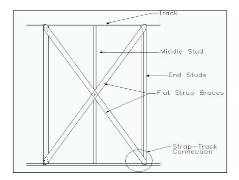
Figure 5.1 General Drawing of Frame with X-bracing.
