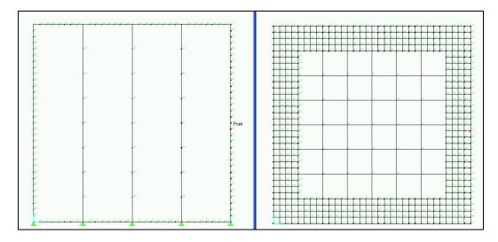
Figure 4.5 Steel Frame and Meshed Shell of Sap2000 model
