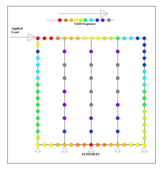
Figure 4.16 Yield pattern for the shear wall with 15 cm screw spacing on center at perimeter. 56
