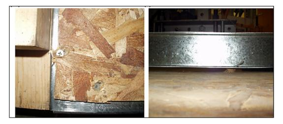
Figure 2.1 Deformation on OSB and screw pulling-out from OSB at tests done by Tian, Wang and Lu (2003)
