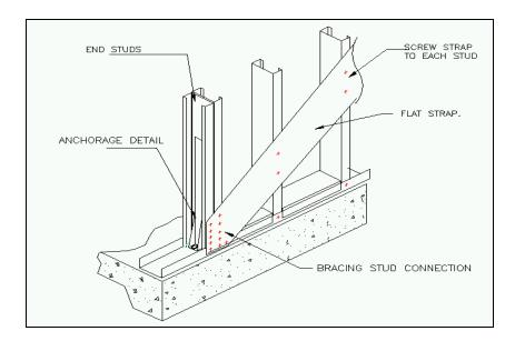
Figure 5.3 Bracing-frame connection detail
