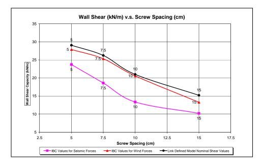
Figure 4.12 Comparison of Nonlinear Link defined Model Nominal Shear Capacity with IBC nominal shear values for wind and seismic forces
