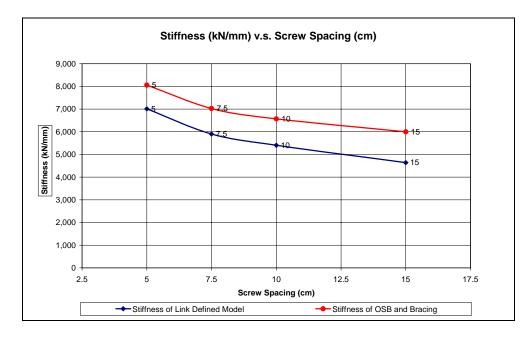
Figure 6.2 Stiffness of Walls vs. Screw Spacing with and without X-bracing
