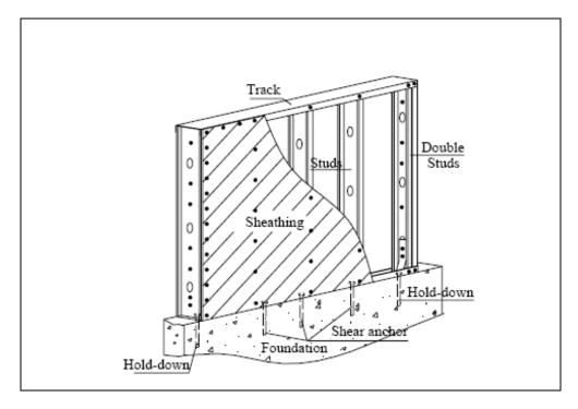
Figure 1.9 Typical Cold Formed Steel Shear Wall, Zhao and Rogers (2002)
