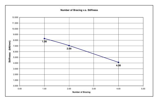
Figure 5.12 Change of Stiffness with Number of Bracing curve
