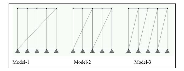
Figure 5.11 Analytical models of shear wall with X-bracing with different number of bracings
