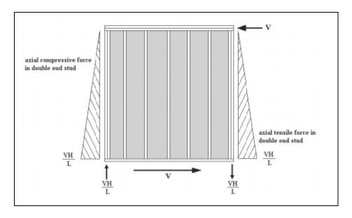
Figure 3.5 Free-Body Diagram of the Shear Walls, Bredel (2003)
