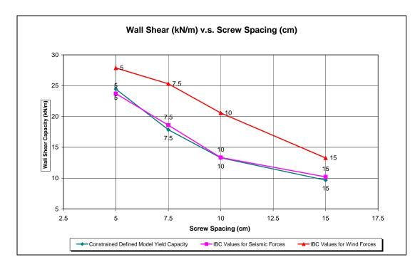
Figure 4.9 Comparison of Constraint defined Model yield Capacity with IBC nominal shear values for wind and seismic forces
