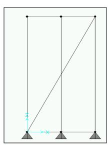
Figure 5.6 Sap2000 model of frame.
