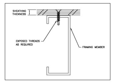
Figure 3.6 Oriented Strand Board and steel stud screw connection, NASFA Publication NT600.
