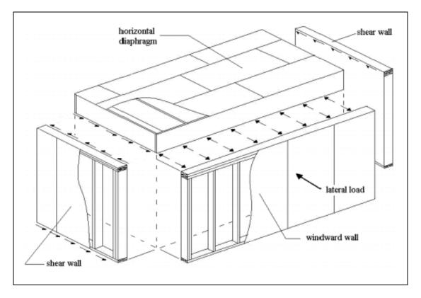
Figure 1.8 Lateral Load Carrying Mechanism of Light framed Building, Bredel (2003)
