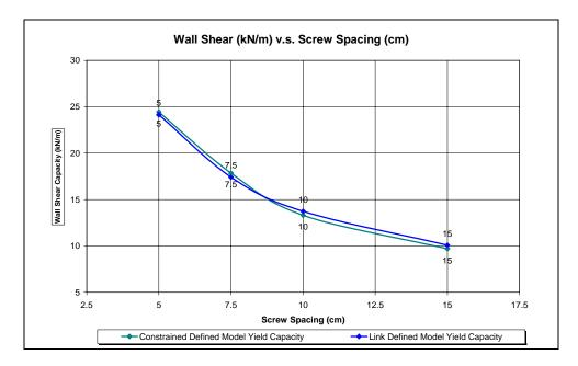
Figure 4.11 Comparison of Nonlinear Link defined Model yield Capacity with Constraint defined Model yield Capacity
