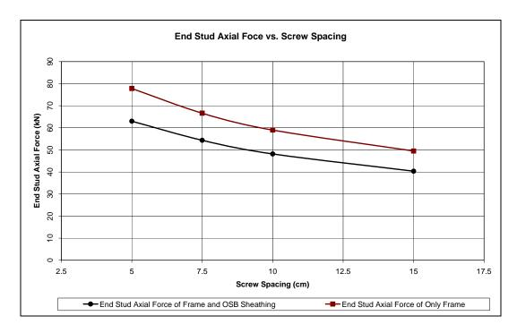
Figure 6.5 End Stud Axial Force vs. Screw Spacing with and without X-bracing
