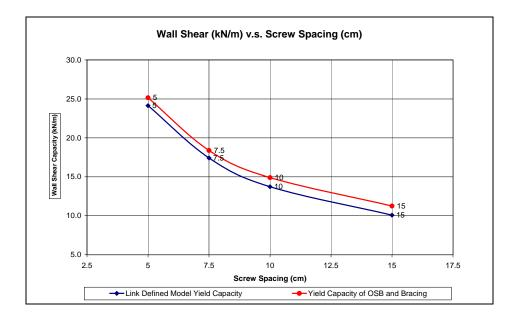
Figure 6.1 Yield Capacities of Walls vs. Screw Spacing with and without Xbracing
