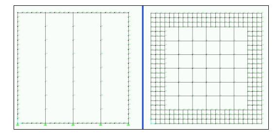
Figure 4.3 Steel Frame and Meshed Shell of Sap2000 model
