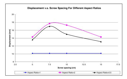
Figure 4.15 Displacement values of frames for different aspect ratios for four different screw spacing
