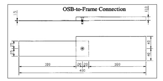
Figure 2.2. Drawing of tested OSB to Steel skeleton connections by Fülop and Dubina (2006)
