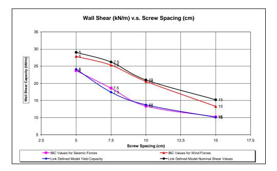
Figure 4.14 Comparison of Nonlinear Link defined Model yield and Nominal Shear Capacity with IBC nominal shear values for wind and seismic forces
