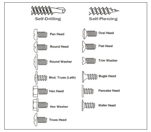
Figure 3.3 Head and Types of screws, Prescriptive Method (2000)
