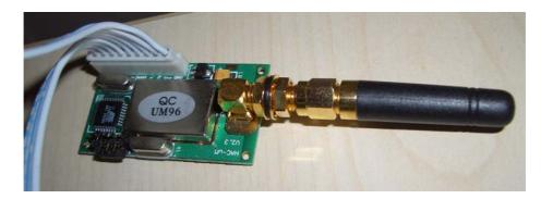
Figure 4.14. Half duplex RF modem.
