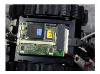
Figure 2.15. One segment of Kohga (Each segment includes a controller.).
