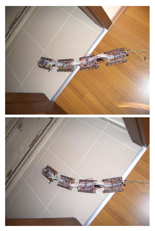
Figure 4.37. Lateral Undulation Gait with Obstacle Avoidance behavior.
