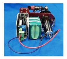
Figure 2.13. Inside of a wheel (Motor, gear head and batteries are included in a wheel system.).
