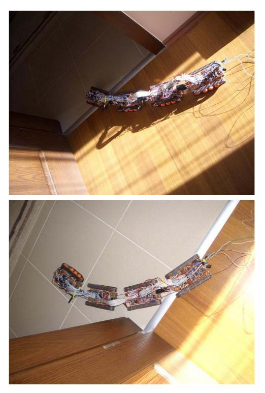
Figure 4.28. Accordion gait. The robot passes through the door way.
