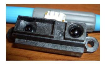
Figure 4.5. SHARP GP2D120 IR range sensor.
