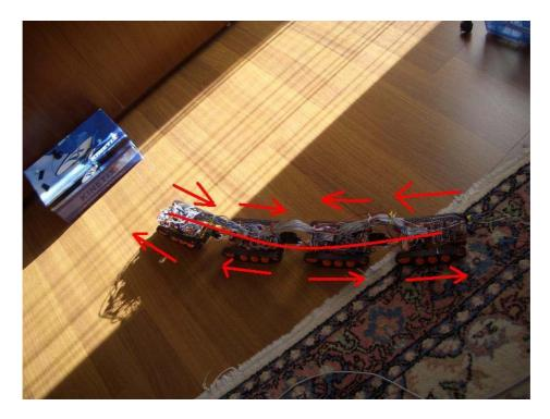
Figure 4.22. The steering of accordion gait. The joint servos are assisted by the palette motion indicated with red arrows.
