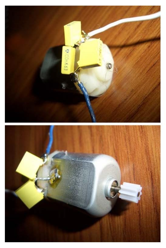
Figure B.1. Shunting of a dc motor. Three 100nF capacitors used. One capacitor is attached between the terminals of the dc motor. Other two capacitors are soldered between the housing and each terminal.
