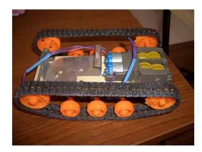
Figure 4.2. Tank Chassis with dc motors and gearboxes.
