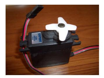
Figure 4.11. Servo used in joints.
