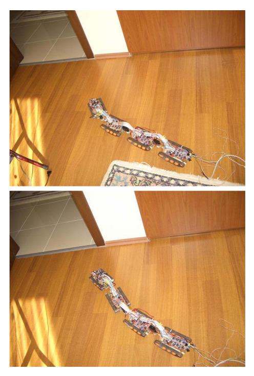
Figure 4.35. Lateral Undulation Gait with Obstacle Avoidance behavior.
