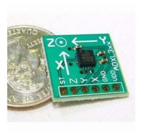
Figure 4.8. Accelerometers with two axes. Accelerometers are positioned to set the +x direction parallel with the corresponding robot segment forward direction. [Picture taken from www.sparkfun.com]
