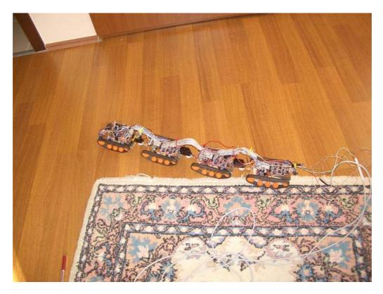
Figure 4.34. Lateral Undulation Gait with Obstacle Avoidance behavior.
