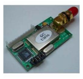
9600 baud half duplex serial connection.
