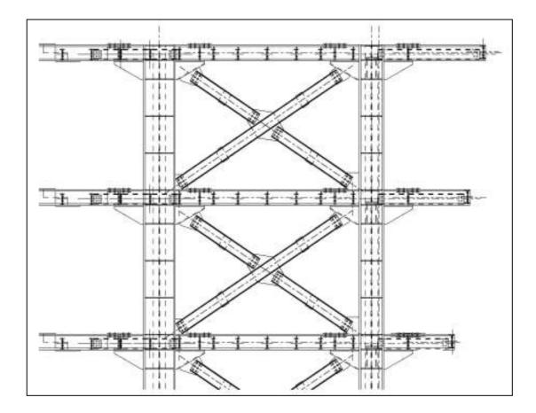
Figure 4.11. The bracings used in the vertical direction
