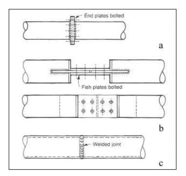
Figure 2.23. Tube-to-tube splice. (Source: Schollar, 1993)
