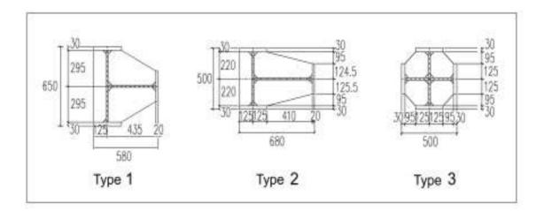
Figure 4.5. Three types of built up sections produced as columns for the TESKOMB Building
