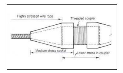
Figure 2.20. Threaded coupling for wire rope sockets (Source: Schollar, 1993)
