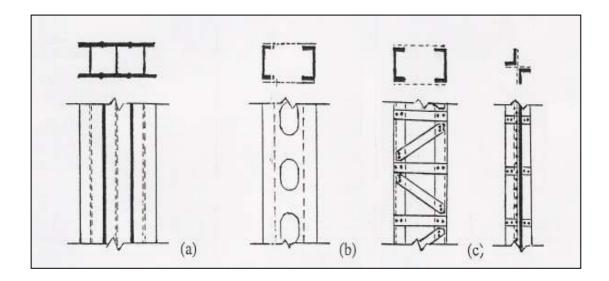
**Figure 2.5.** Built-up columns; (a) solid wall column, (b) solid wall column with perforated cover plates and (c) open type column (Source: Keyder, 1993)
