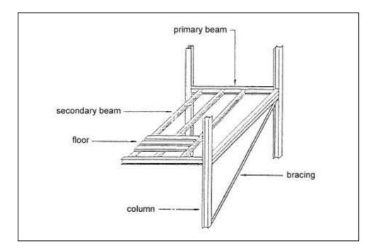
Figure 2.4. Typical components of a steel frame (Source: Hart, 1992)
