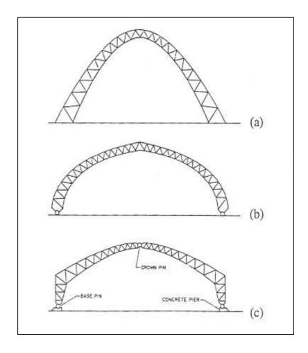
Figure 2.25. Typical steel arches; (a) hingless arch,
