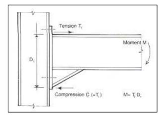
Figure 2.18. Beam-to-column moment connection using a gusset (Source: Schollar, 1993)
