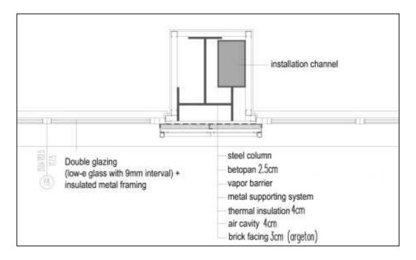
Figure 4.23. A detail showing the installation channel adjacent to the steel column
