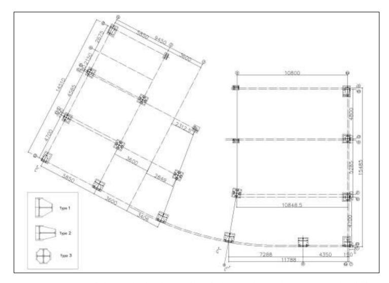
Figure 4.4. Structural plan showing location and sizes of columns and beams (Source: Rona Mühendislik)
