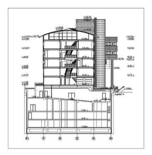
Figure A.2. Section BB of TESKOMB Building (Source: Uz Mimarlık)
