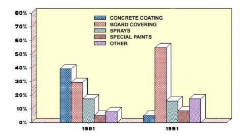
Figure 2.42. Fire proofing methods used for steel framed structures in England (Source: Akbay, 2006)
