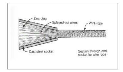
Figure 2.19. Diagram of splaying out of wire rope (Source: Schollar, 1993)
