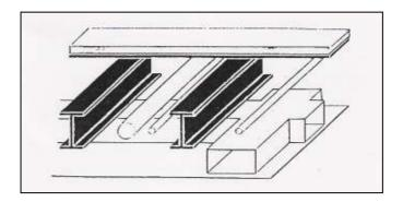
**Figure 2.11.** Lateral zoning (Source: Copeland, Glover, Hart, Hayott and Marshall, 1983)
