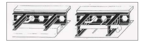
**Figure 2.10.** Unimpeded routing of services (Source: Copeland, Glover, Hart, Hayott and Marshall, 1983)
