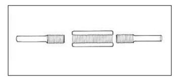
Figure 2.21. Threaded coupling for bars
