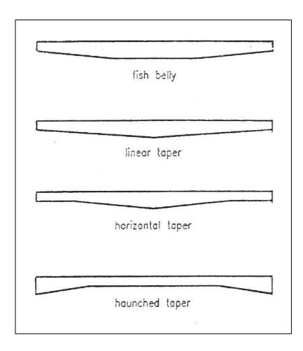
Figure 2.7. Tapered beams (Source: Berktin, 1994)
