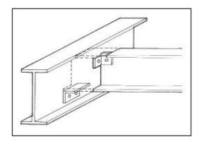
Figure 2.17. Beam-to-girder connection using seating and restraining cleats. (Source: Thomas, 2003)
