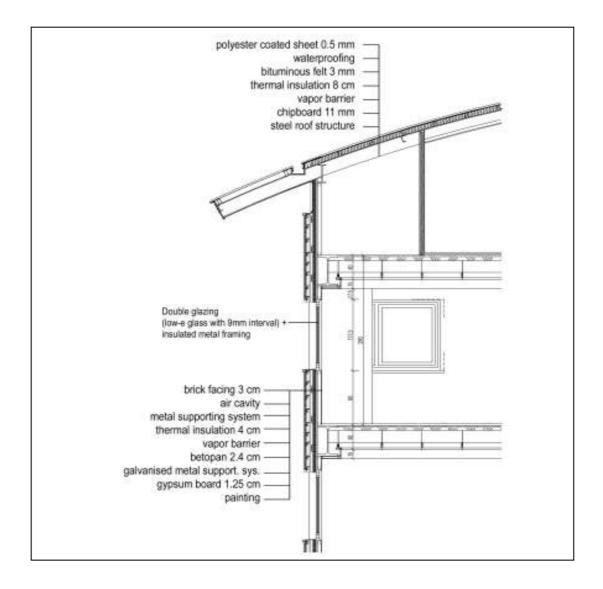
Figure 4.21. Detail drawing of the building
