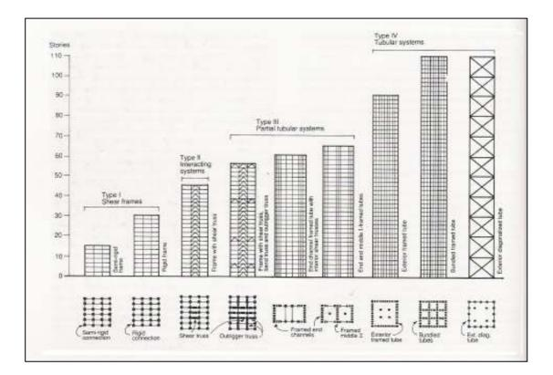
Figure 2.29. Comparison of structural systems (Source: Iyengar, 1993)
