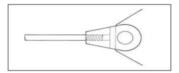
Figure 2.22. Pin joint connection for bar (Source: Schollar, 1993)
