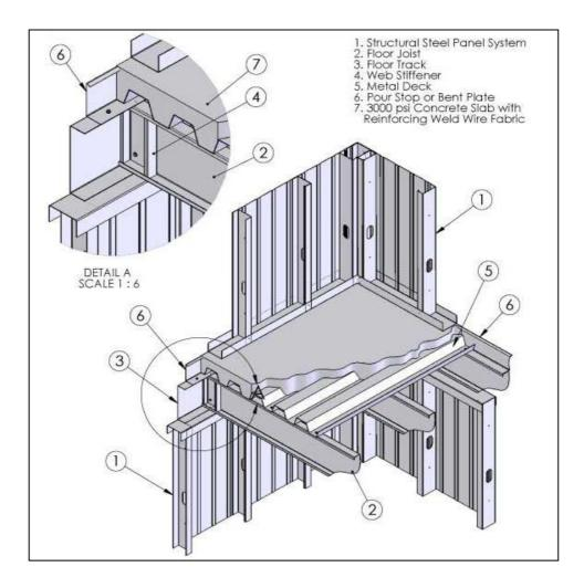
**Figure 2.9.** Steel deck floor system (Source: www.nexgenhomes.net, retrieved 2006)
