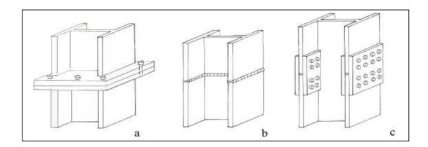
Figure 2.14. Direct compression in a column joint carried by (a) end plates, (b) on welds, and (c) on splice plates (Source: Schollar, 1993)
