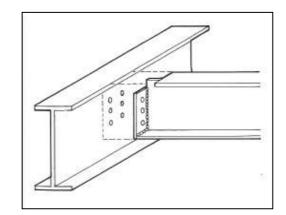
Figure 2.15. Beam-to-girder connection using web cleats (Source: Thomas, 2003)
