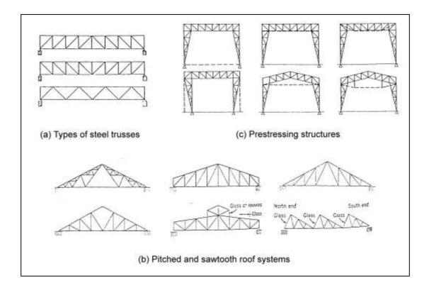
Figure 2.24. Structural systems for single-storey structures (Source: Watson, 1986)
