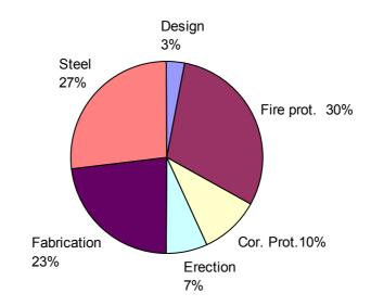
Figure 2.38. Pie chart showing cost breakdown for steel construction projects (Source: Latter, 1985)
