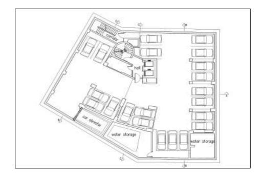
Figure 3.6. Third basement floor designed as a garage
