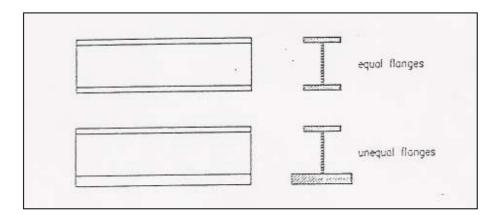
Figure 2.8. Fabricated plate girders (Source: Berktin, 1994)
