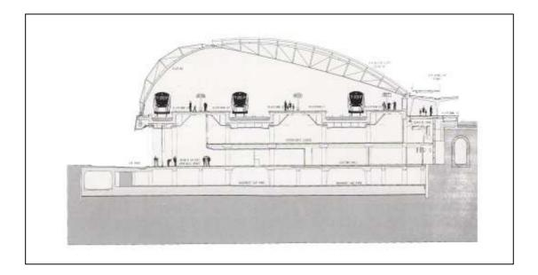
Figure 2.26. Cross-section of the Channel Tunnel Terminal Building in London, England (Source: Plank, 1993)
