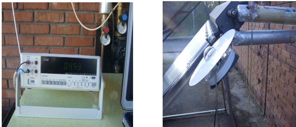
Figure 4.5 Views of the pyranometer and the milivoltmeter.
