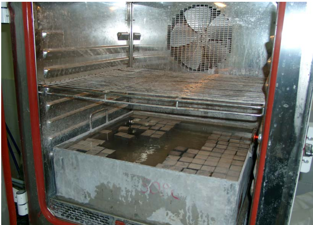
Figure 4.6 Climatic Chamber Where Different Curing Regimes Were Applied
