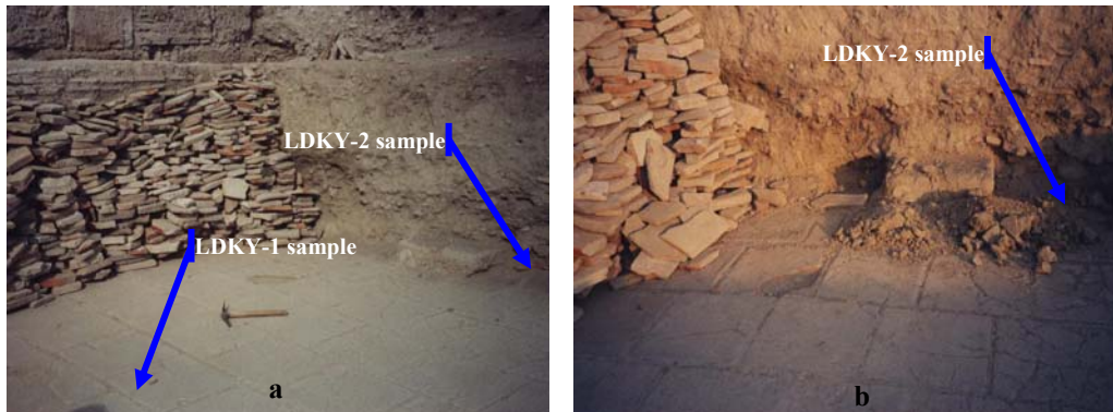
Figure 3.1(a, b) Ceramic floor tiles of the room which is at the right side of North of the front church door entrance. (LDKY-1: ceramic floor tile which was exposed to the sunlight, LDKY-2: ceramic floor tile which was not exposed to the sunlight.)
