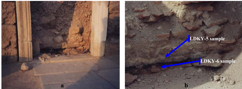
Figure 3.3(a, b) Ceramic ceiling tiles which were taken from the entrance of the church door. (LDKY-5 and LDKY-6 are the ceramic ceiling tiles which were not exposed to sunlight but they were in a fire layer and hence were exposed to heat.)
