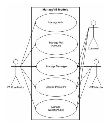
Figure A37 Use case diagram of "Manage VE" module
