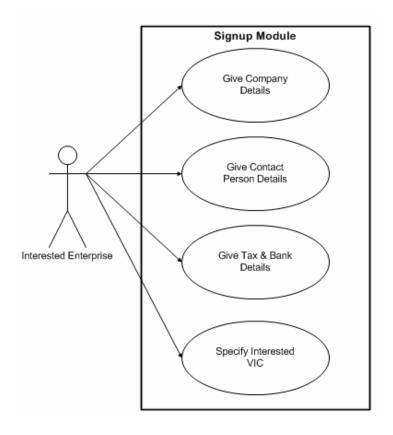
Figure A18 Use case diagram of "IE Signup" module
