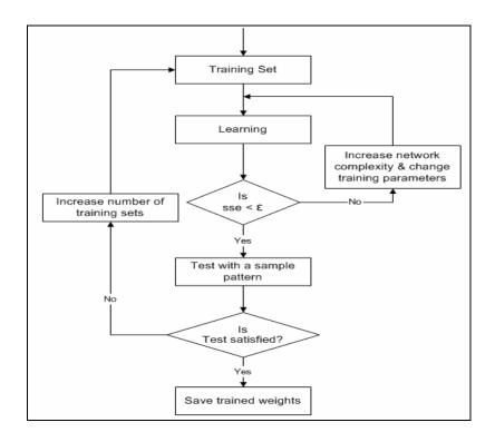
Figure 6.38 Training and testing procedure of neural network
