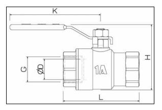
Figure 7.3 Dimensioning ball valve for general use
