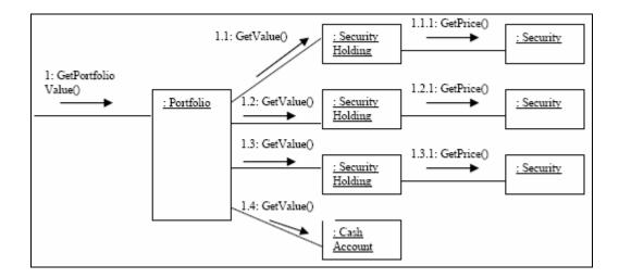
Figure 2.16 Collaboration diagram for the calculation of the value (Rational, 1997)
