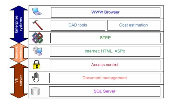
Figure 6.1 Layered ICT architecture for VE system
