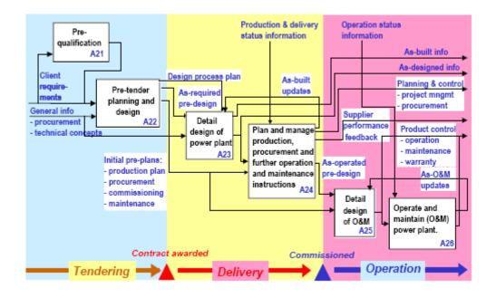
Figure 2.8 Functional model of power plant construction (Valikangas et al, 2000)
