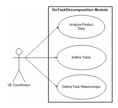
Figure A21 Use case diagram of "Task Decomposition" module
