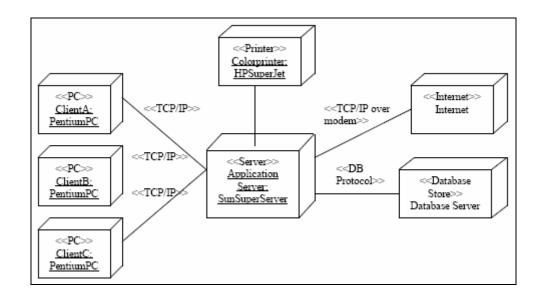
Figure 2.20 Deployment diagram of physical hardware (Rational, 1997)
