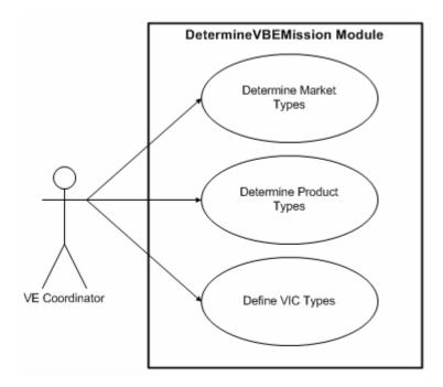
Figure 6.11 Use case diagram of "Determine VBE Mission" module
