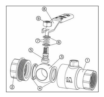
Figure 7.2 Assembly view of ball valve for general use
