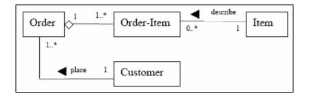
Figure 2.12 Class diagram for modeling an order (Rational, 1997)
