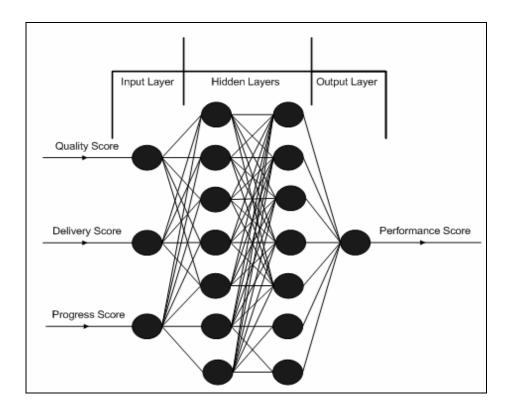
Figure 6.37 Fully connected multi-layered neural network
