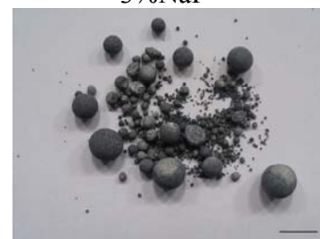
Figure 72 Magnesium droplets for the experiments involving the effect of NaF (length of the line is 1 cm).
