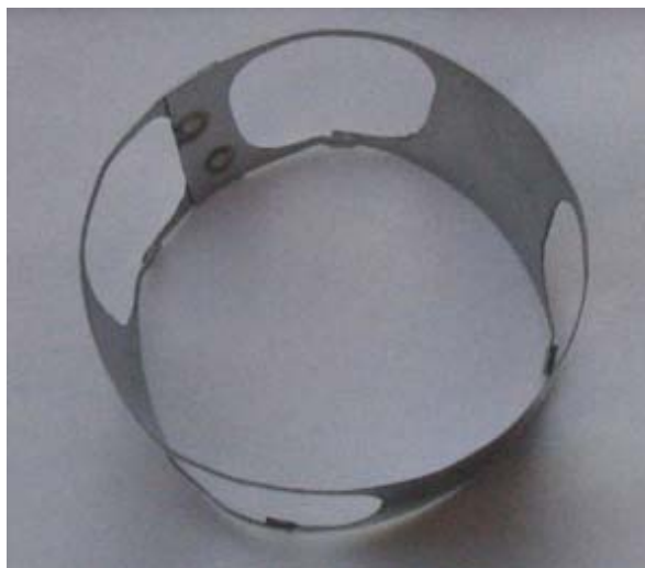
Figure 24 Stainless steel cathode without extension rod.
