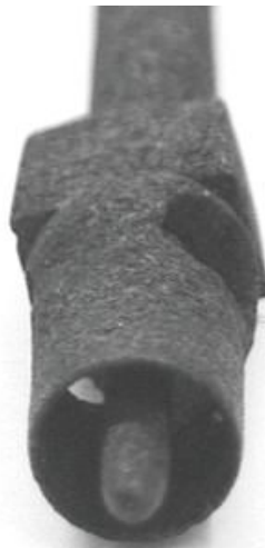
Figure 23 Graphite anode with its extension rod.
