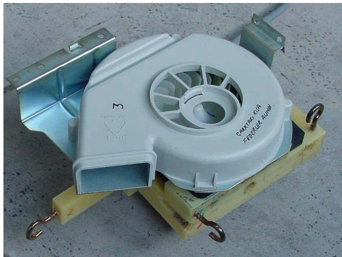
Figure 5.2 Fan motor noise suppressing box
