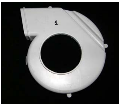
Figure 4.7 Volute with inlet modification
